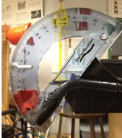
Figure 75: Second image of displacement test of original TEE CCW pitch
