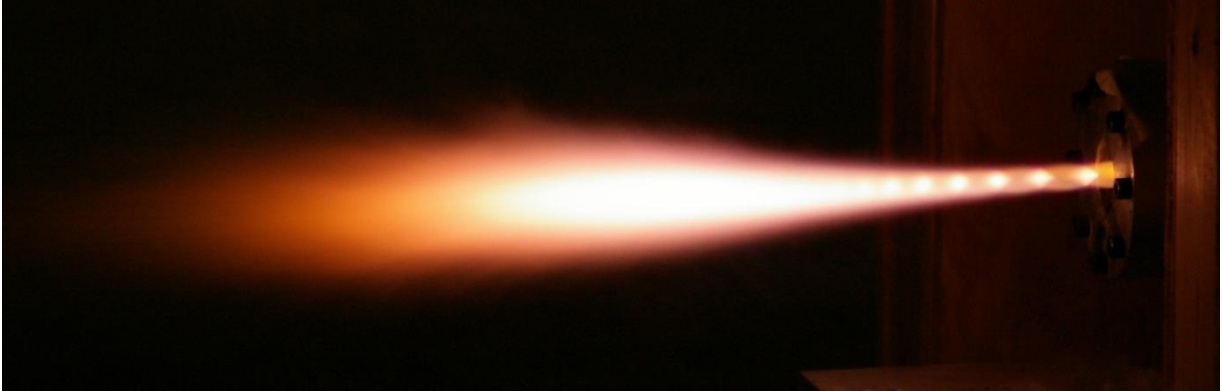
Figure 92: Exhaust Plume From 50N Paraffin Motor with 4 Port Injector, Test 14b
