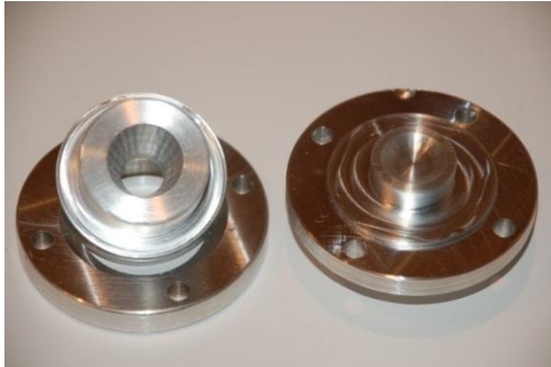
Figure 43: Nozzle Holder and Injector after machining. Three inch OD Retention rings shown with each for scale.
