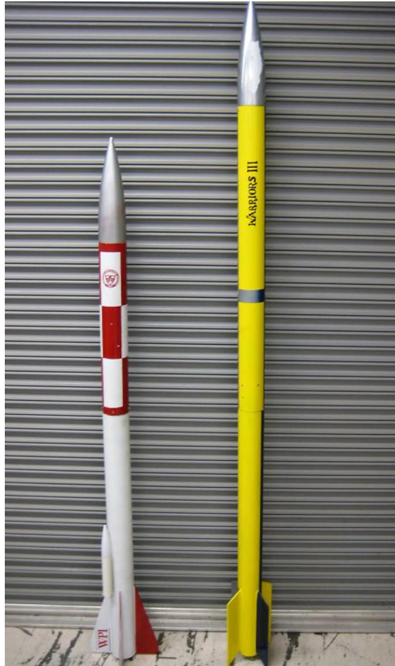
Figure 19: Assembled Test Rockets Rocket Height: Left -65.3 in., Right – 79.2 in.
