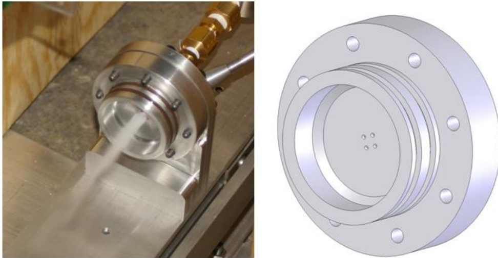
Figure 47: Initial flow testing of the four port injector and CAD model showing four port arrangements
