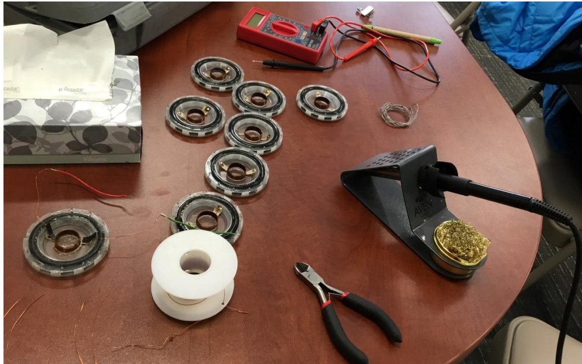
Figure 3: Coil cut and glued
