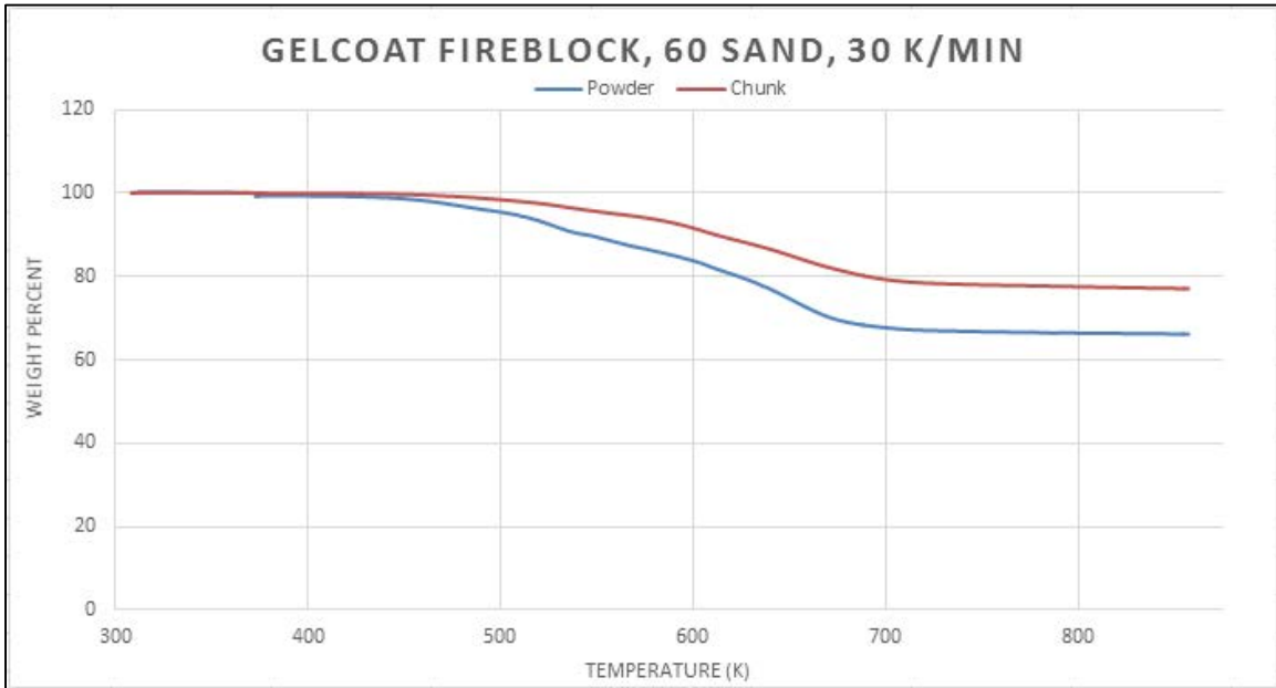
Figure 89: Powder, chunk, and drop samples single heating rate method at 30 K/min
