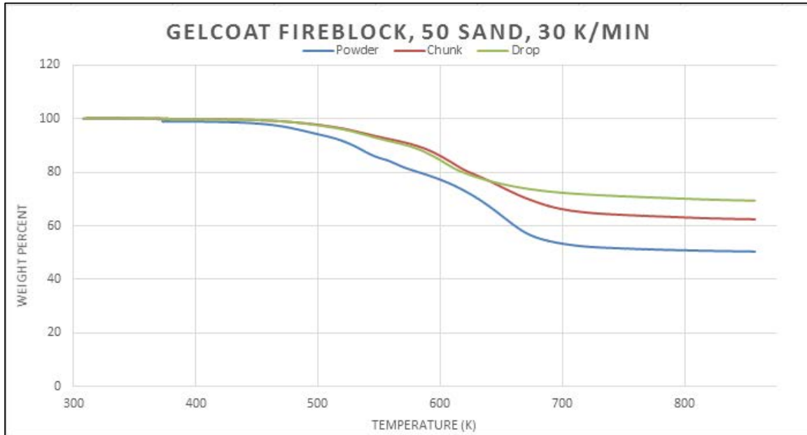
Figure 83: Powder, chunk, and drop samples at single heating rate, 30 K/min
