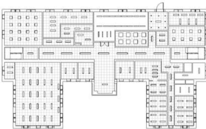
Figure 23 Lighting fixture layout of the second floor
