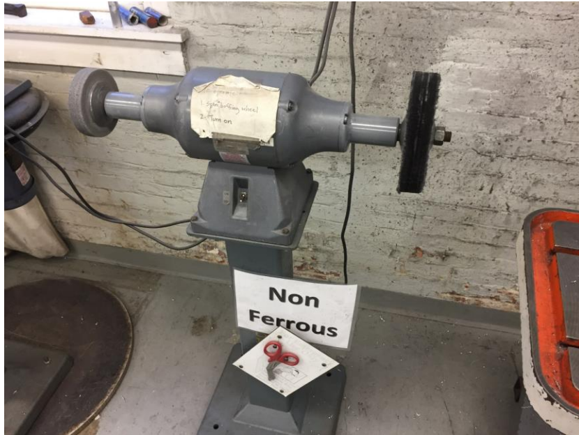
Figure 83: Non-Ferrous Buffing Wheel for Surface Finish.
