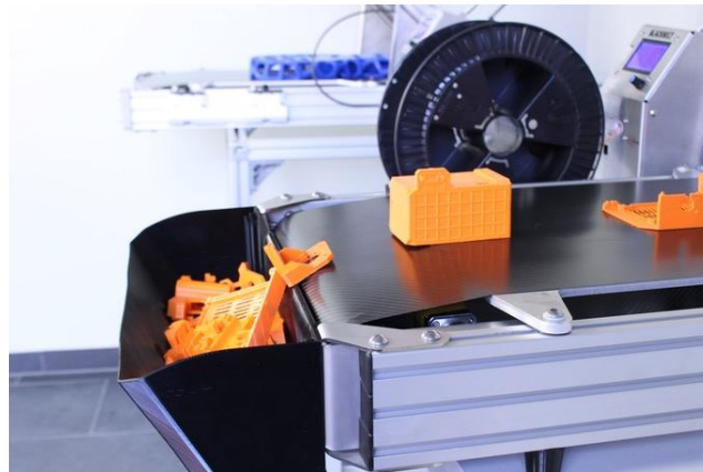
Figure 21: Automatic Removal on the Blackbelt 3D Printer [39].
