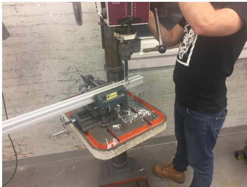
Figure 60: Drilling Notches for the Pulley Inserts
