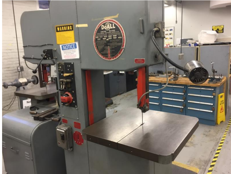
Figure 87: Vertical Band Saw in Washburn Shops.
