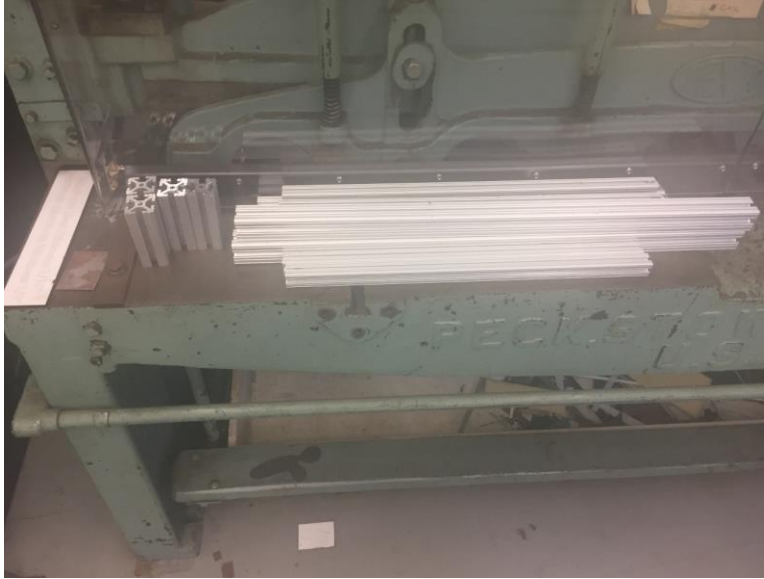
Figure 59: Final Band Saw Cuts for 8020 Framing.
