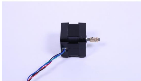
Figure 3: Hobbed Gear and Motor Assembly [9].
