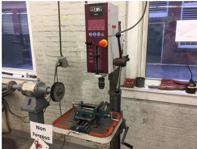
Figure 86: Drill Press with Different RPMs based on Orientation of Levers.
