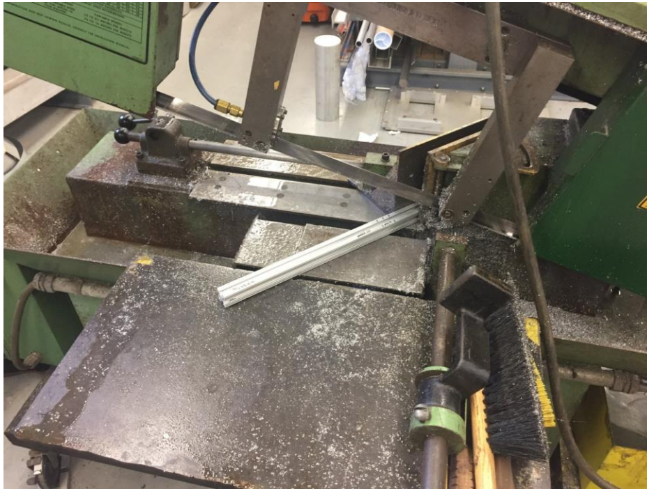
Figure 58: Preparation of the Angled Cut.
