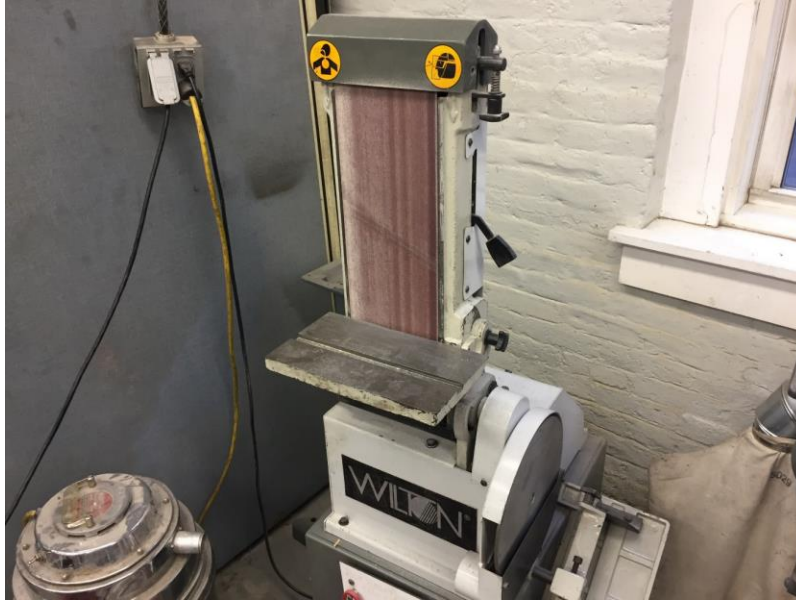
Figure 91: Belt Sander in Washburn Shops.
