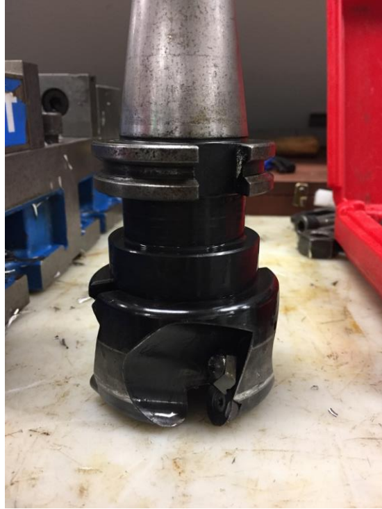
Figure 93: Face mill Tool for Facing Parts.
