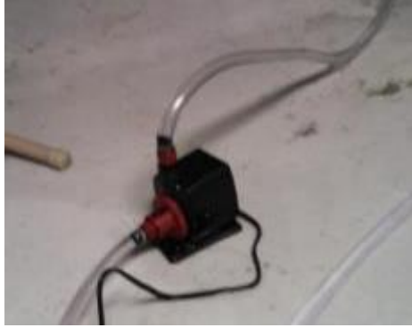
Figure 12: Hydor Seltz pump circulating water from the tank through heat exchanger.
