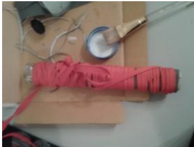
Figure 42: Wrapped Handle Assembly, Left to Dry Overnight.
