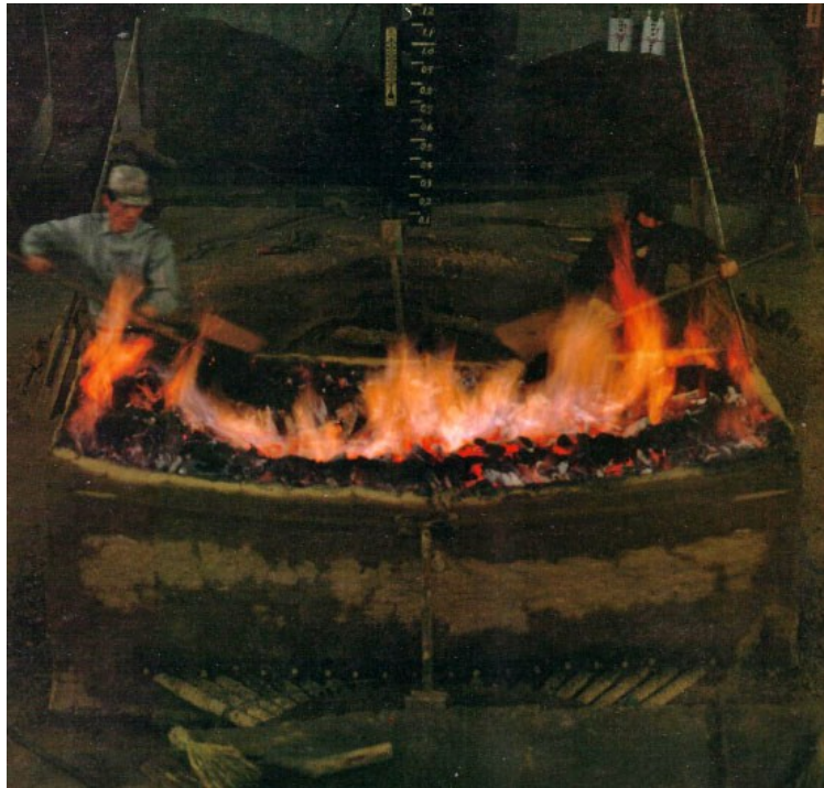
Figure 5: Tatara Furnace Burning Iron into Tamahagane Steel.
