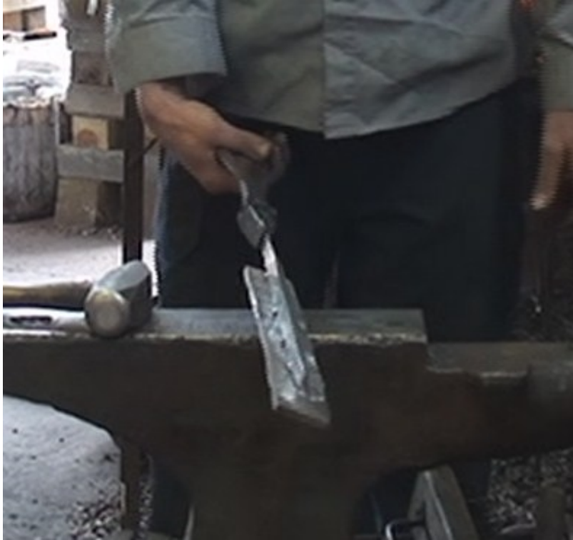
Figure 33: Joined 1018 Steel and 1095 Steel.
