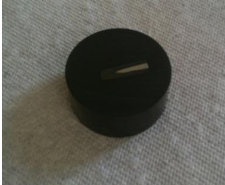
Figure 45: Etched & Mounted Blade Sample.
