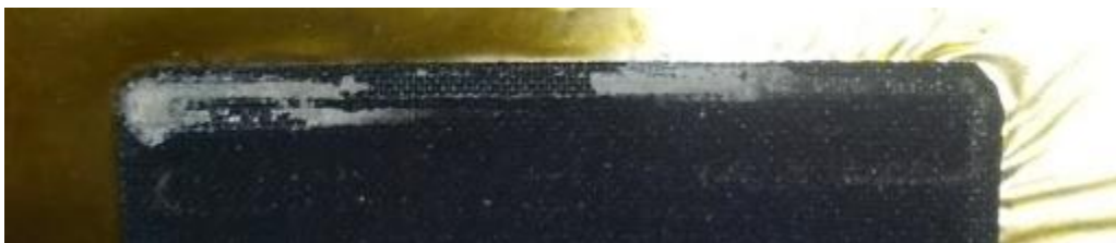
FIGURE 23: BLOCKAGE OBSERVED ON THE GAS DIFFUSION LAYER OF THE MEMBRANE ELECTRODE ASSEMBLY.
