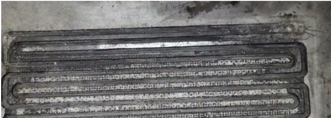
FIGURE 25: BLOCKED SERPANTINE CHANNELS IN THE GRAPHITE PLATE
