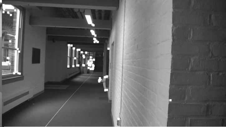
Partial Derivative Threshold Detection overlayed on Original Image
