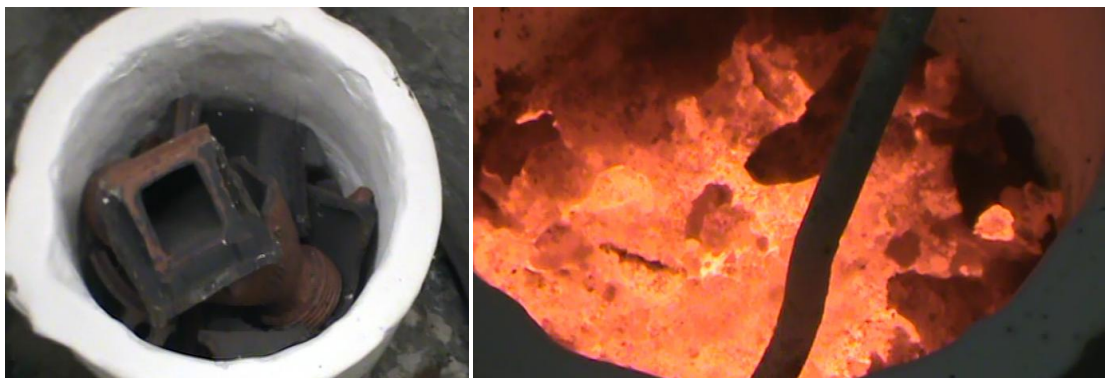
Figure 52: Bronze Pieces Placed Inside Crucible within Furnace (Before and After).
