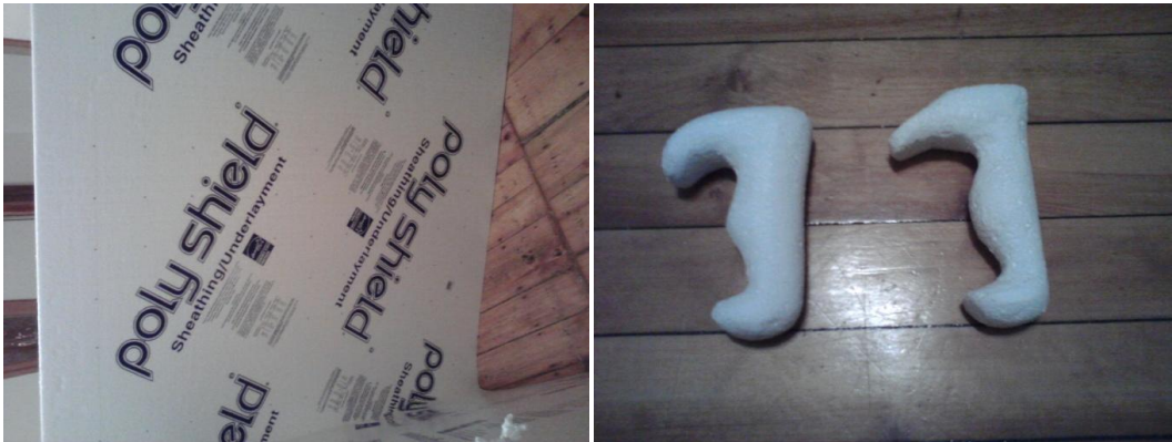
Figure 50: Handles Carved out of Polystyrene (Practice Run).
