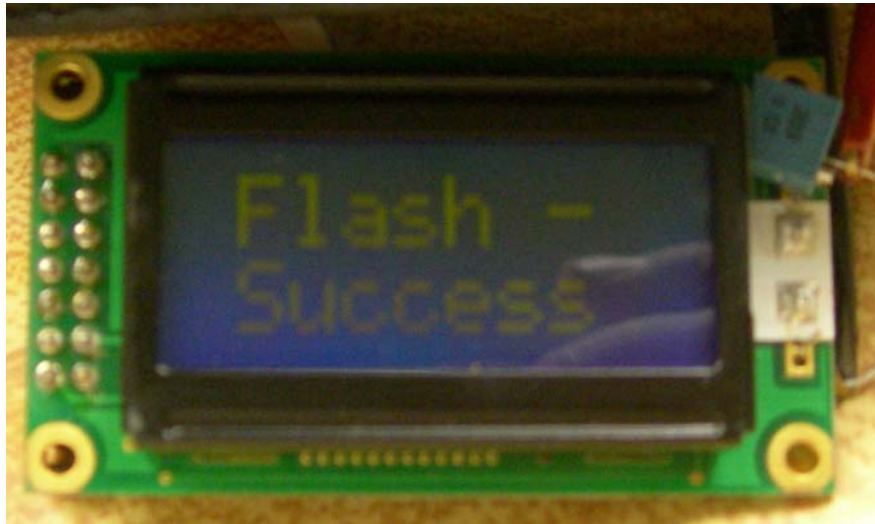
Figure 52: Memory Testing - "Flash_Success"
