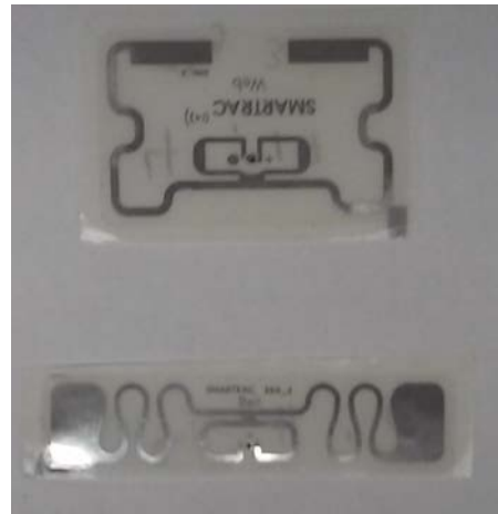
Fig 2.2 Flexible label Passive RFID tag
