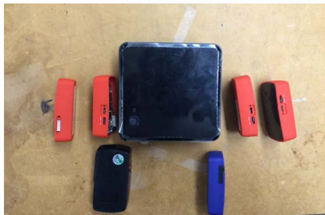
Fig. 2.7 Showing the Ultra Wide-Band System. The black box is the Base station( Black box), the fixed nodes(Orange nodes), the bridge node(black node), and the mobile node(blue node).
