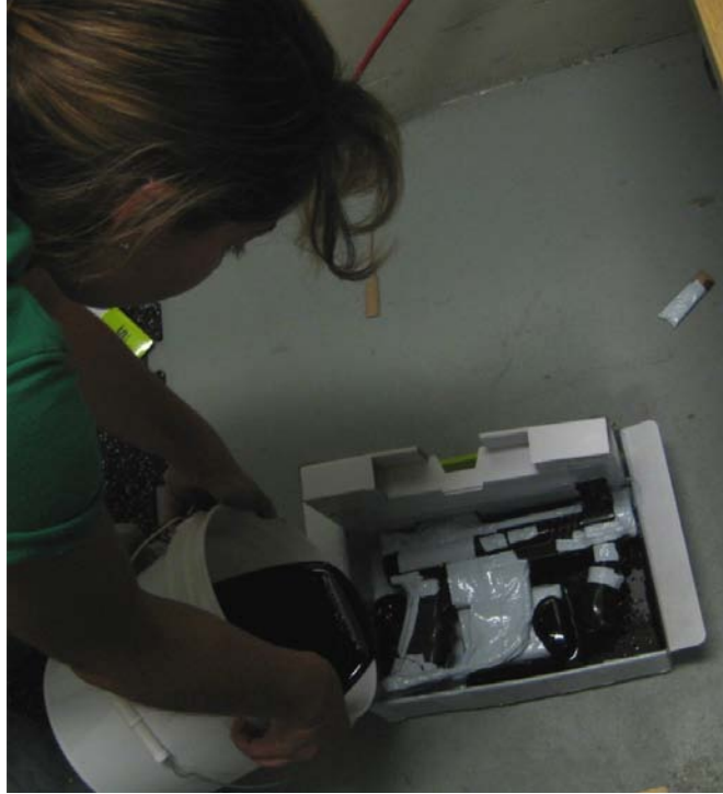
Figure 35: Pouring of the Urethane Casting Compound into the Prepared Mold
