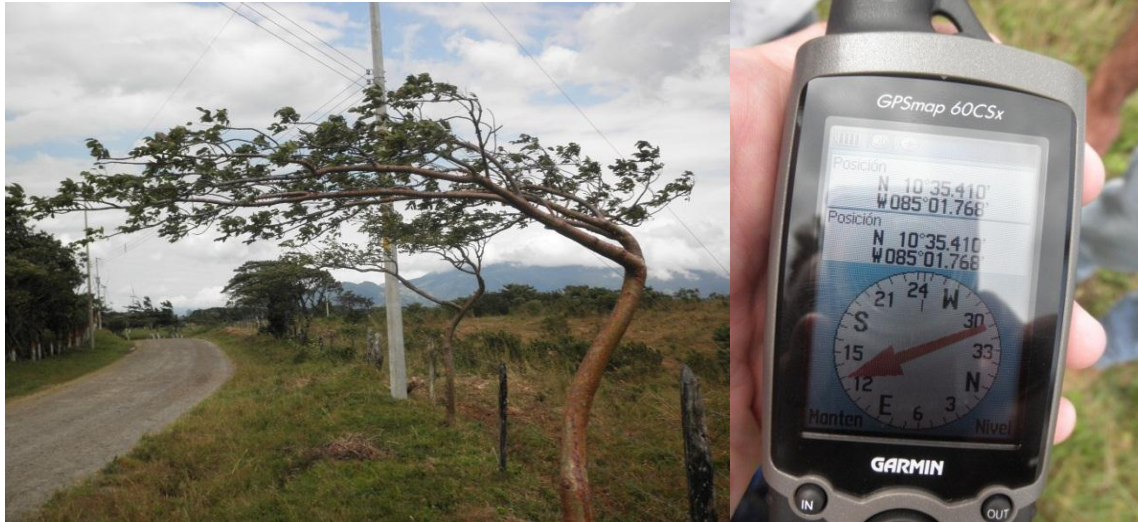
Figure 4.3 PEVA flagging tree (left) and compass in the direction of flagging (right)
