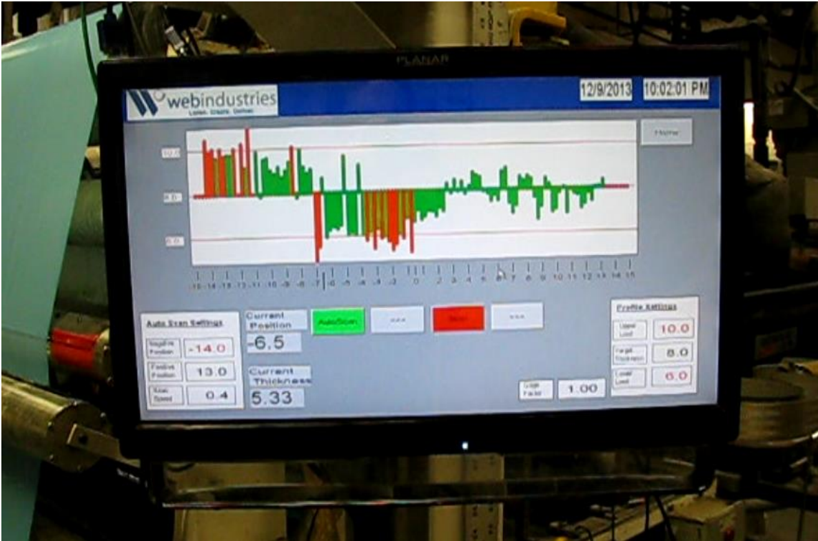
Figure 67. This picture shows the touchscreen monitor mounted on the MX ergotron wall mounted monitor arm. The monitor is displaying the thickness profile of a 30" wide web.
