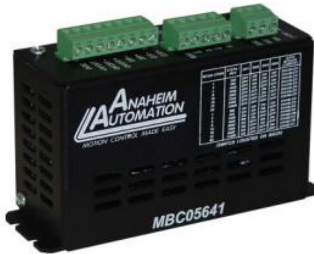
Figure 15. The MBC05641 stepper drive takes 24-48V, and provides adjustable current from .5 to 5A and adjustable steps using DIP switches [13].
