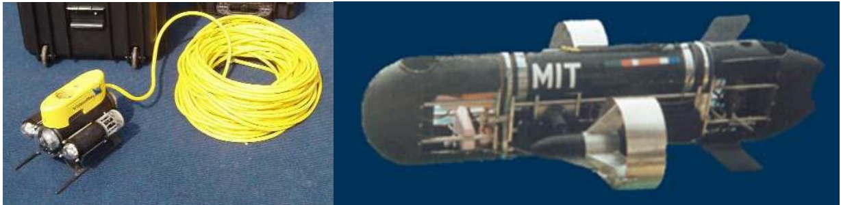
Figure 1: An ROV (left, has tether) and AUV (right, no tether)
