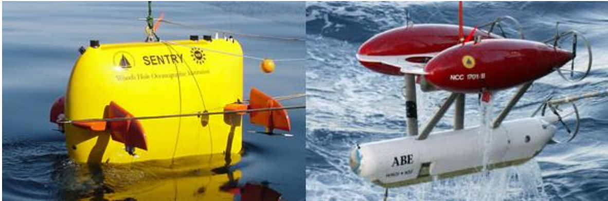
Figure 3: Non-Torpedo Shaped AUVs: SENTRY (left) and ABE (right)
