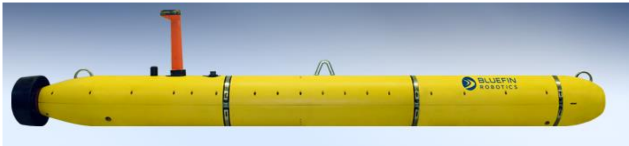
Figure 2: Bluefin-12S - A typical Torpedo Shaped AUV
