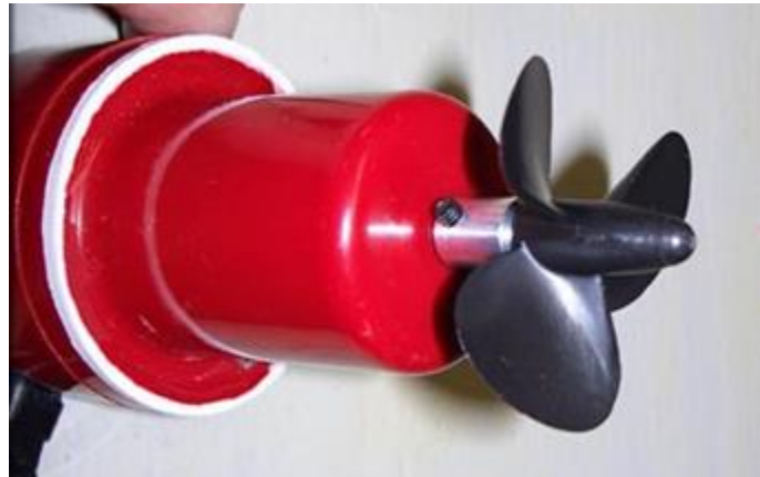
Figure 38: Modified Rule 1100 GPM Bilge Pump
