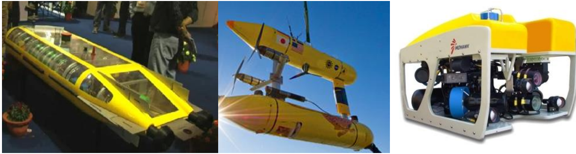
Figure 5: Pressure Vessel (left) , Flooded Shell (middle) and Open Frame (right) AUVs.
