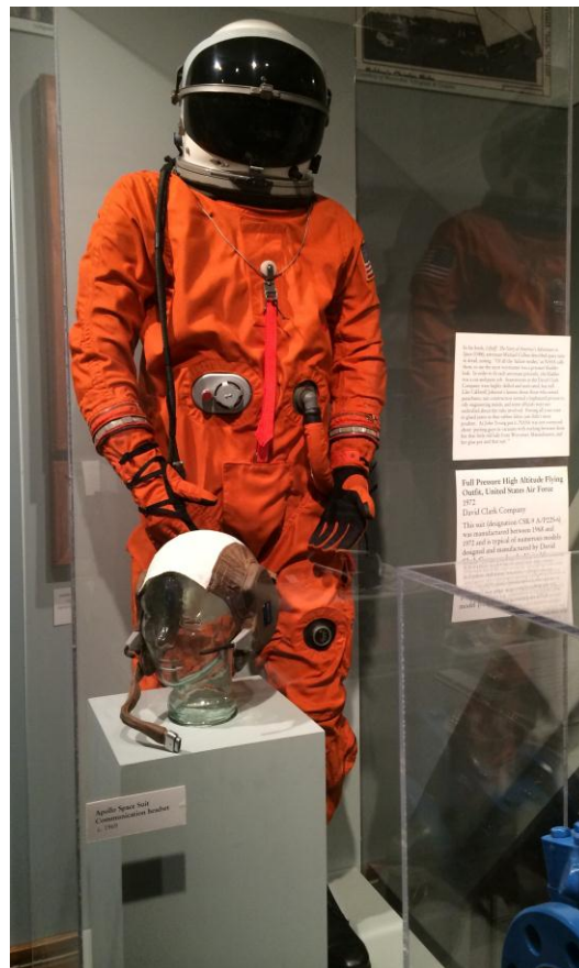
Figure 15: Full Pressure High Altitude Flying Outfit made by the David Clark Company (Photo Credit: DellaGrotte, 2014)
