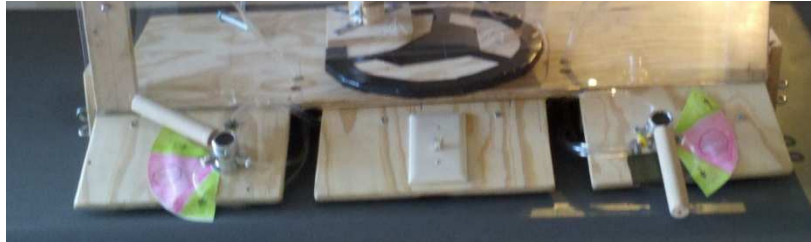
Figure 6 Interface panels fixed on a slant and valve and light switch layout
