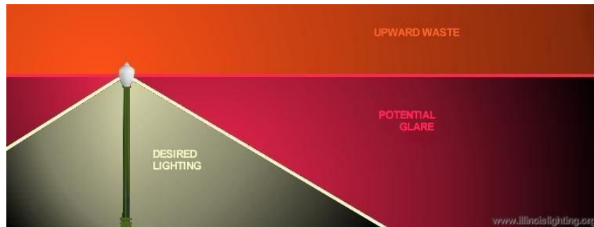
Figure 2: Diagram of light trespass. The section labeled “desired lighting” is the only beneficial light being emitted from the lamp. The purple area represents “potential glare” and the orange section represent “upward waste” which is a major contributor to sky glow. http://www.illinoislighting.org/fixture1.html
