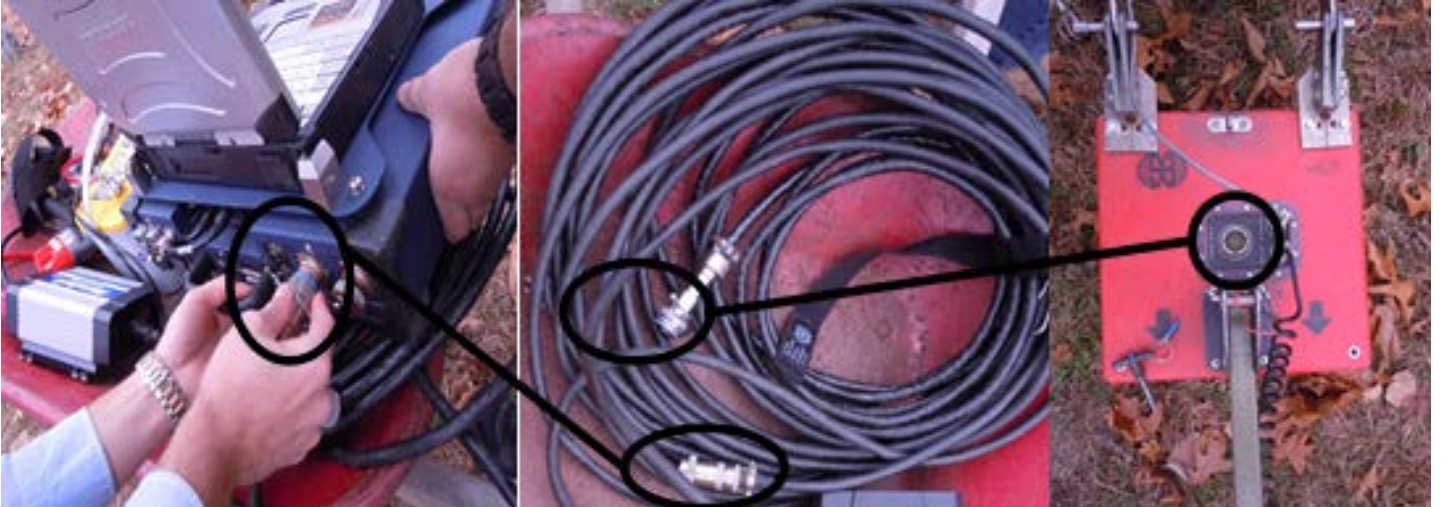
Figure 6: Connecting laptop to antenna
