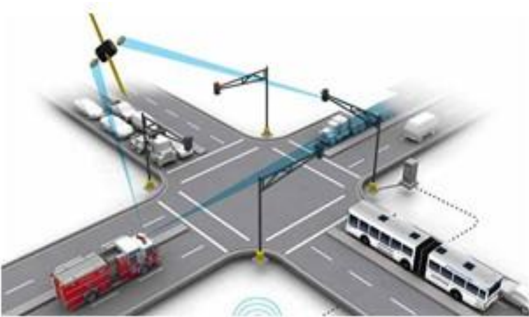
Figure 27: A GPS-based preemption system (US Department of Transportation [80])
