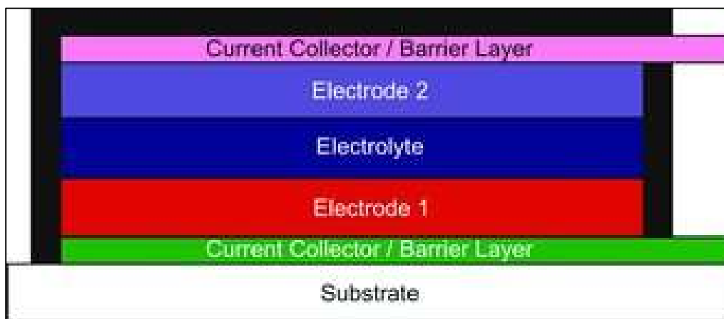
Figure 9: Demonstration of a Generalized Construction of All-Solid-State Li Ion Batteries 34
