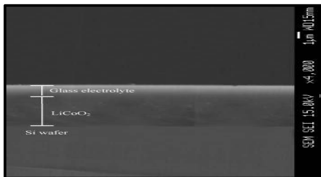
Figure 13: SEM of Solid-State Electrolyte Layers Deposited Through Aerosol Deposition 40
