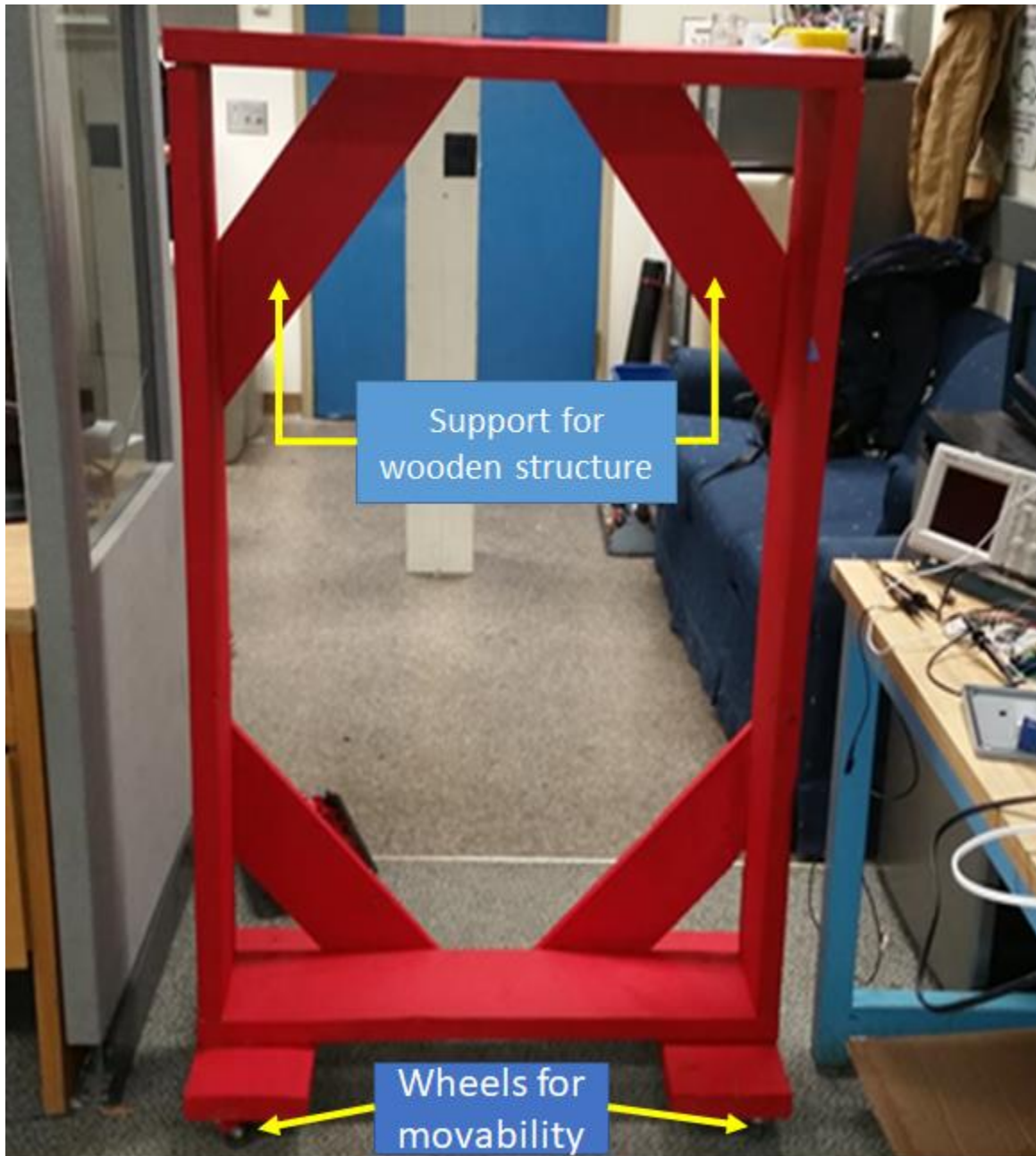
Figure 90: Wooden Structure Used to Handle All Components of the Autonomous Bus System. The wooden structure was designed to be mobile and support the implemented design. A shelf was added to hold the acrylic box holding all of the necessary components and to provide a mounting point for the PIRs.
