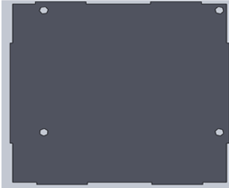
Figure 85: Solidworks Model of Bottom Casing Part with Four Hole Cutout Features. The dimensions for this part are 7.50" x 7.50". The four holes are for the standoffs needed for the Zedboard.
