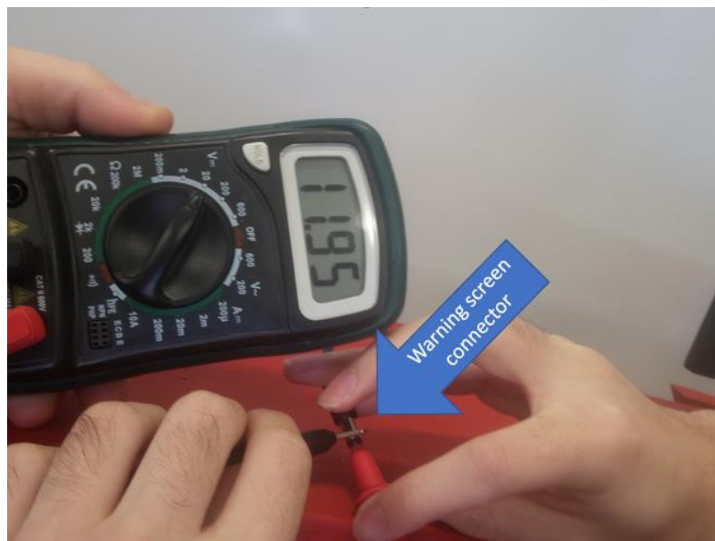
Figure 80: Testing the RC Jack for the Warning Screen. The output was roughly 12 volts. The red probe was connected to the inner diameter while the black probe was connected to the outer diameter of the RC jack.
