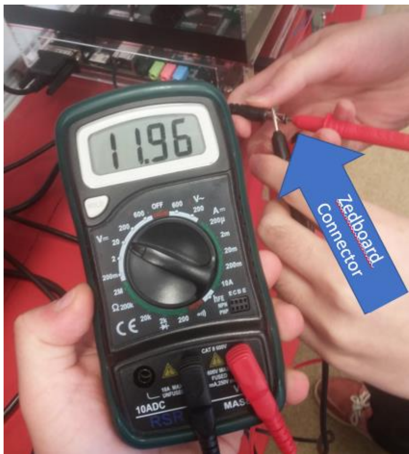
Figure 78: Testing the RC Jack for the Zedboard. The output was roughly 12 volts. The red probe of the multimeter was inserted into the inner diameter of the RC jack while the black probe was connected to the outer diameter.
