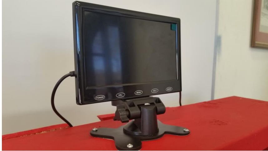
Figure 39: 800x480 resolution VGA screen that was used to display a visual alarm. Screen turns green (No Danger), yellow (Danger Warning zone) or red (Critical Action zone) based on the location of the object.
