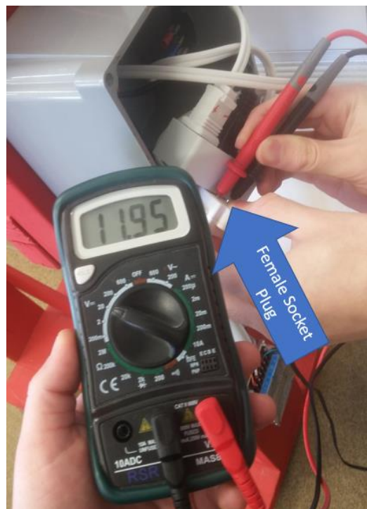
Figure 76: Testing the Female Socket Plugs from the Extension Cord Running from the Power Supply. It provided roughly 12 volts. The red multimeter probe was connected to the positive terminal of the female socket plug and the black probe was connected to the negative terminal.
