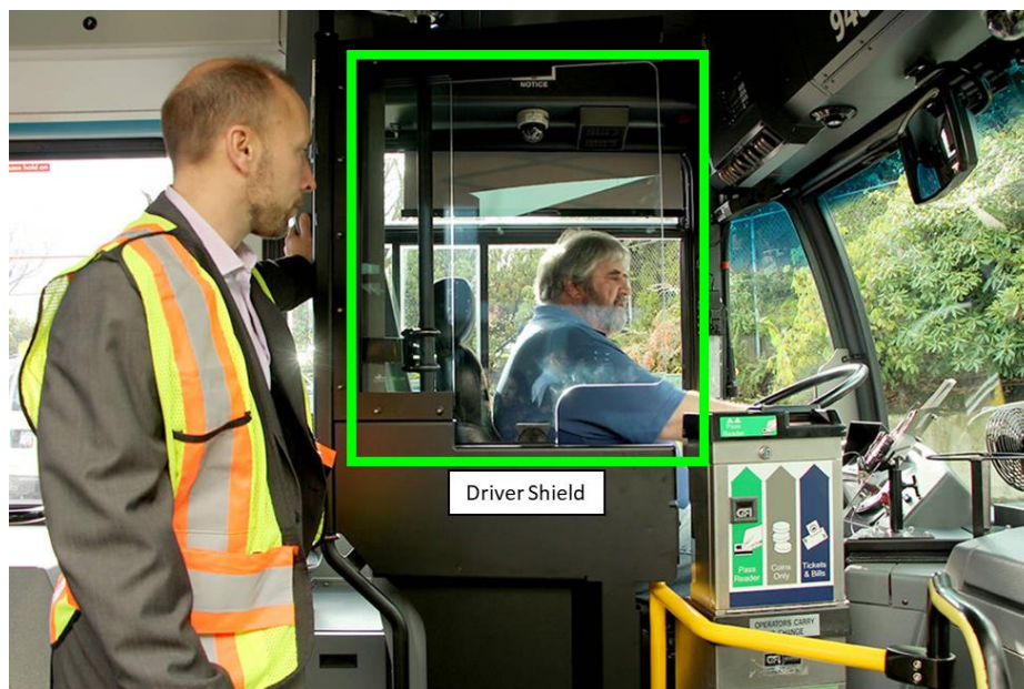
Figure 6: Shield Installed as a Means to Protect Bus Drivers from Pedestrians. The shield is highlighted in green. These shields are usually constructed from strong plastic to withstand hits without worry of shattering. Potential issues with the shields include glare and feelings of claustrophobia, which may turn drivers away from using them. [24]
