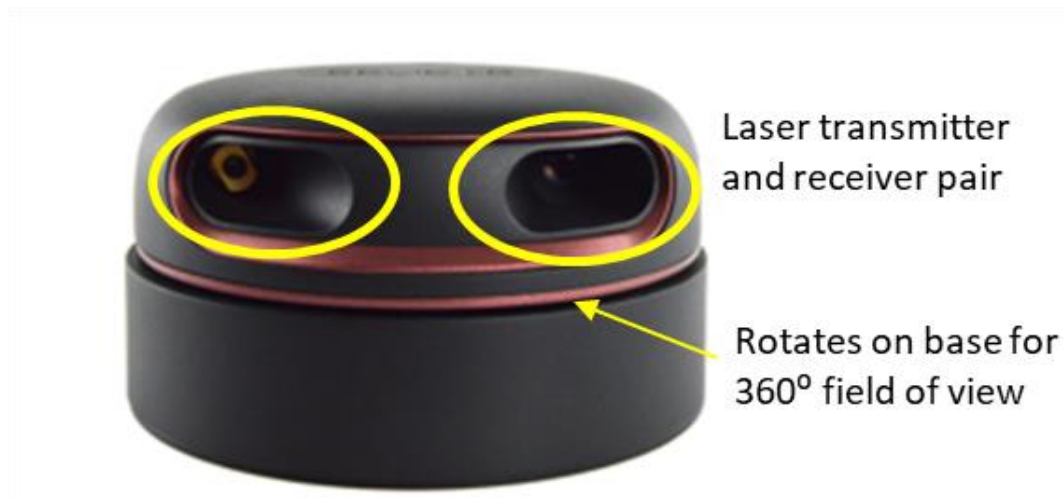
Figure 13: RPLIDAR A2 LIDAR Sensor. The sensor features a laser transmitter and receiver for determining object distance through reflections. The sensor's housing is able to rotate 360 degrees on the base for maximum field of view. [79]
