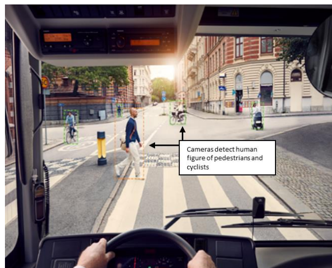
Figure 8: Volvo Pedestrian & Cyclist Detection System. This system monitors the bus's surroundings using cameras and alerts the driver when action needs to be taken. [9]
