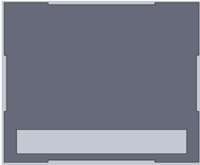
Figure 84: Solidworks Model of Casing Side Part with Rectangular Cutout. The dimensions of the cutout are 6.50" x 7.50". A cutout of 1" x 5.67" was made to help manage airflow and for accessibility to the Zedboard.
