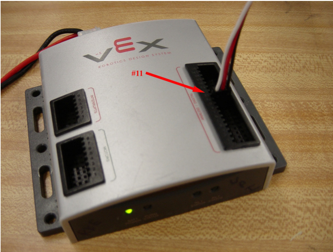
Figure 53 - Image of the VEX controller and wire from the solenoid wire, noting order of the colored wires and port number of the connection
