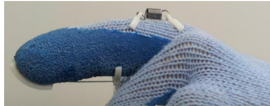
Figure 16 | Spring-cable actuated glove prototype. The cable allows for active flexion and the spring provides limited extension upon release of cable
