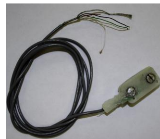
Figure 9 | Custom EMG surface electrode developed at WPI.
