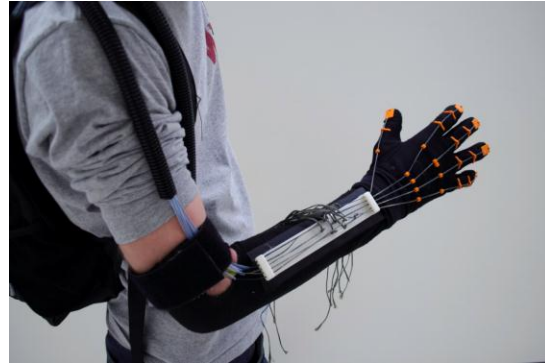
Figure 34 | Forearm cable guides serves as the connection point between glove and Bowden system. Here the cables can be adjusted for individual tension. Note there is one on the dorsal side of the arm and one
