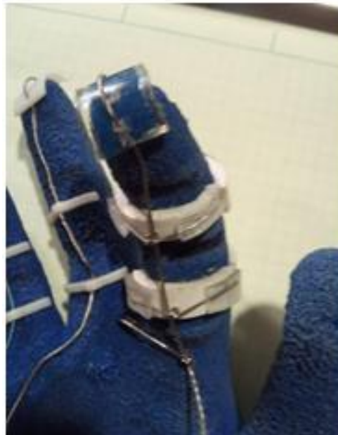
Figure 21 | Proof of concept set-up: wire secured via PVC rings on a garden glove. This demonstrated that cable tension was capable of actuating the finger. Note this glove was merely used for testing.
