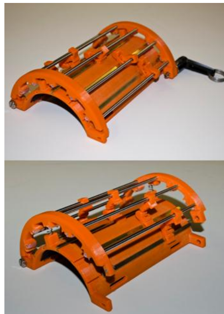
Figure 33 | Quick release mechanism locked (top). Pin released (bottom).
