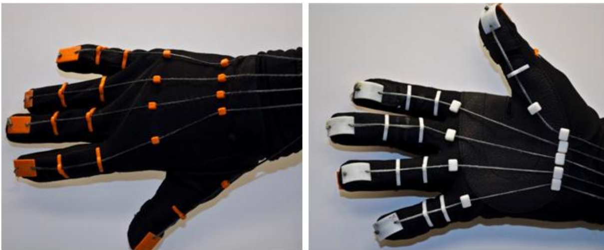
Figure 23 | Final cable guide assembly on glove. Cable lines run centered down the middle of the long axis of each digit and are attached rigidly at the fingertips. Note fingertip, phalanx, and palmar guides.
