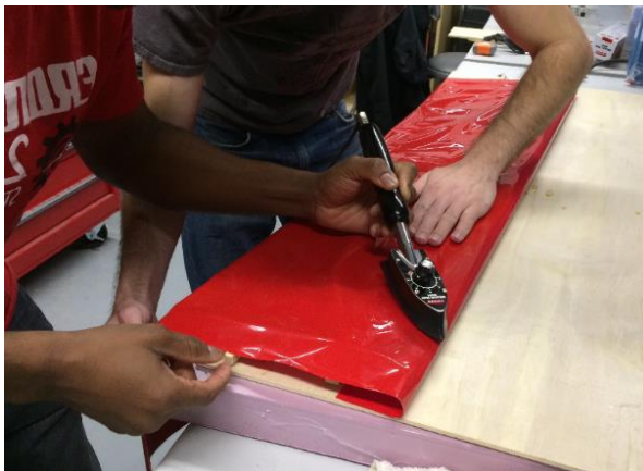
Figure 7.3 - Applying MonoKote Shrink Wrap (left); 3D Printed Bottle Case (right)
