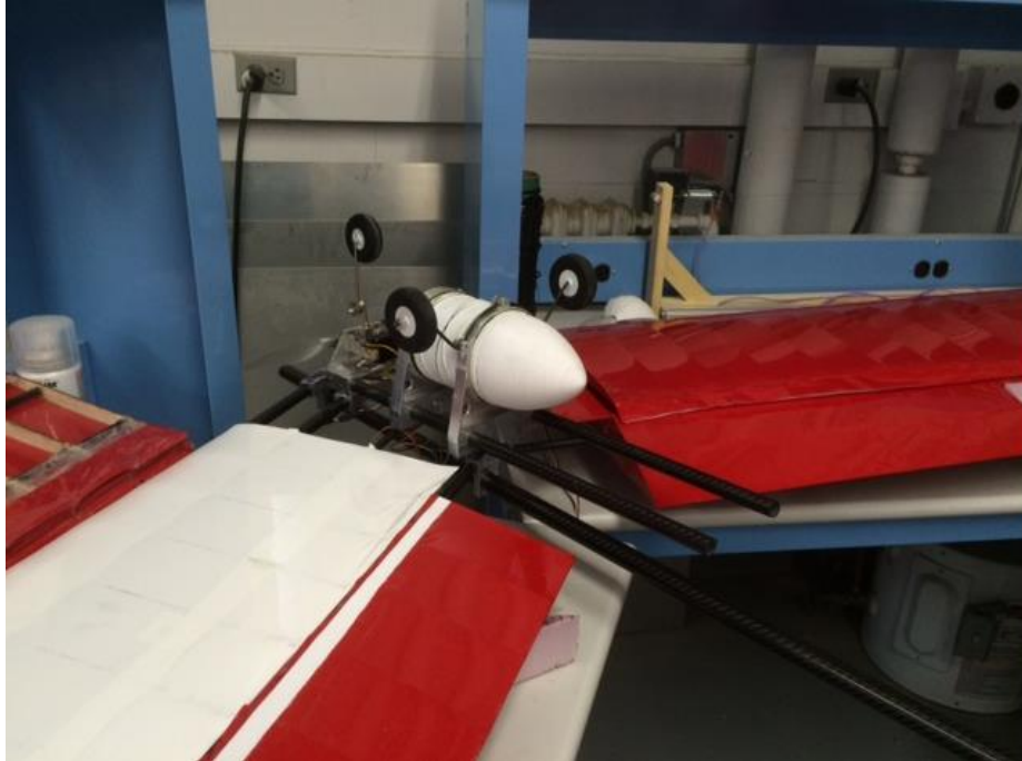
Figure 7.6 - Production Aircraft with Landing Gear Mounted Inversely in the Manufacturing Support Aircraft
