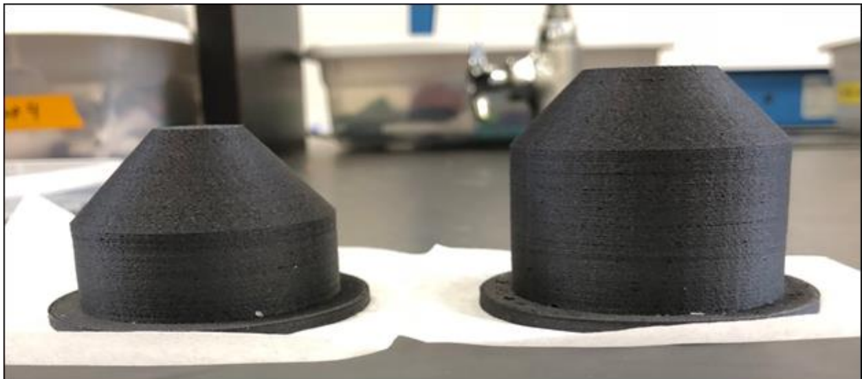
Figure 23. Printed HIPS/20% AC filters of Design A (left) and Design B (right).
