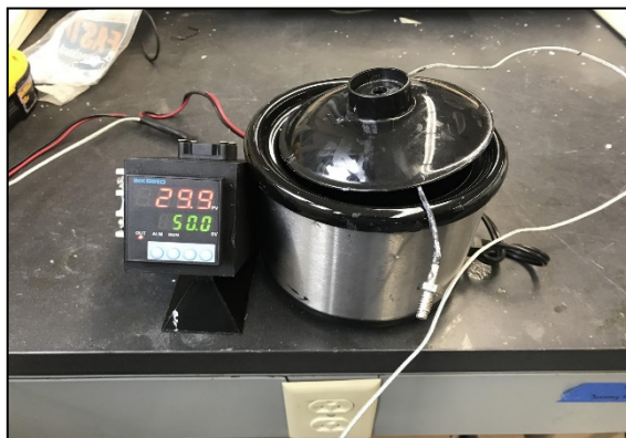
Figure 8. A proportional-integral-derivative (PID) controlled heater used for combining raw materials.
