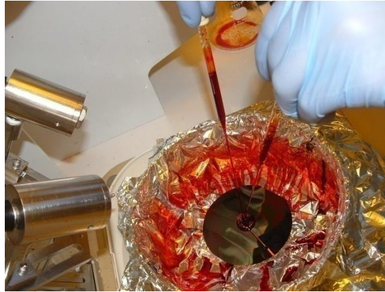
Figure 38 - Spin Coating Photoresist Application Technique
