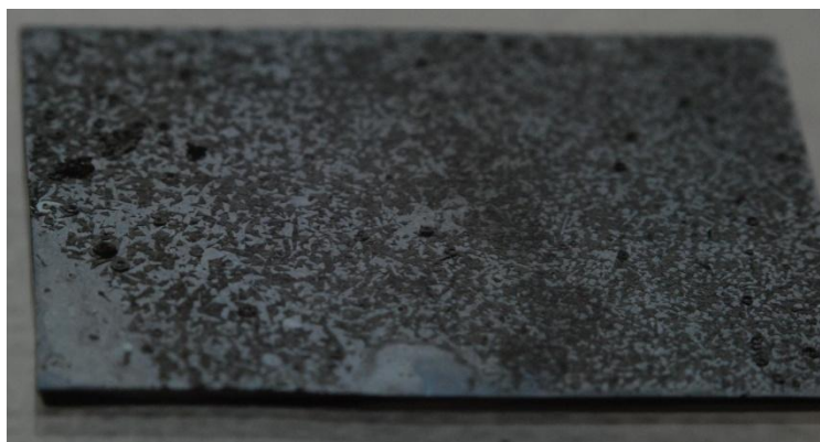
Figure 24 - An Example of an Obliterated Wafer
