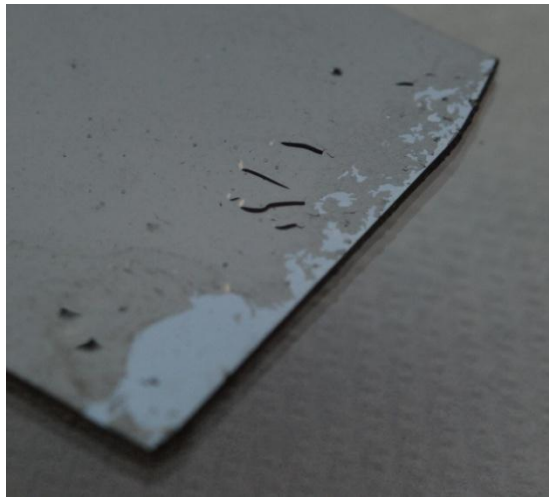
Figure 21 - Wafer Displaying a "Cracking" Result
