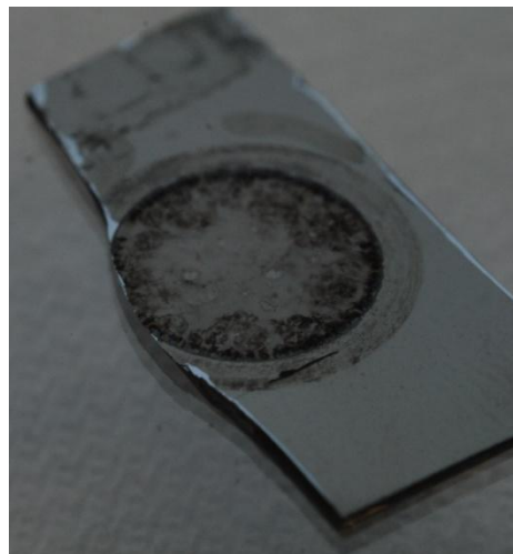
Figure 25 - An Example of Electrically Unstable Carbon Wafer
