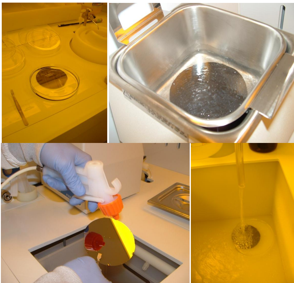
Figure 35 - Spin Coating Liquid Cleaning Treatment
