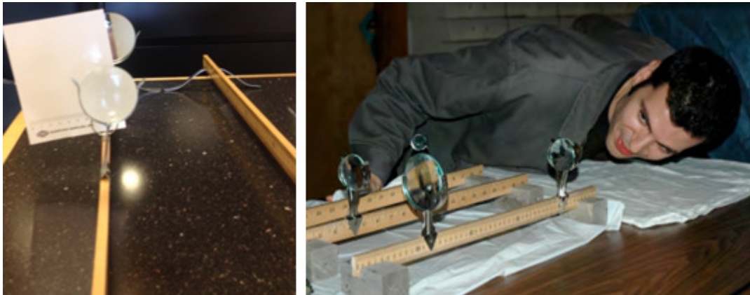
Figure 9: Place the magnifier on the meter-stick section on the opposite side of the screen of the larger lens. Lean down to look through the lens at the image on the screen. Now remove the screen and look through the magnifier, called the eyepiece, because it's what we look through with our eye.
