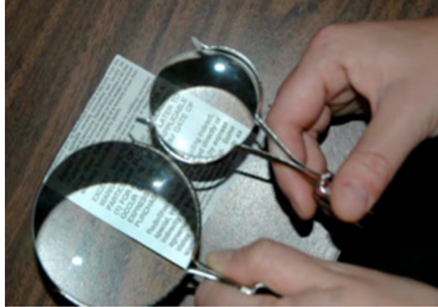
Figure 5: Hold the 50mm diameter 200mm FL lens (thinner) and the 75mm diameter lens over the paper.
