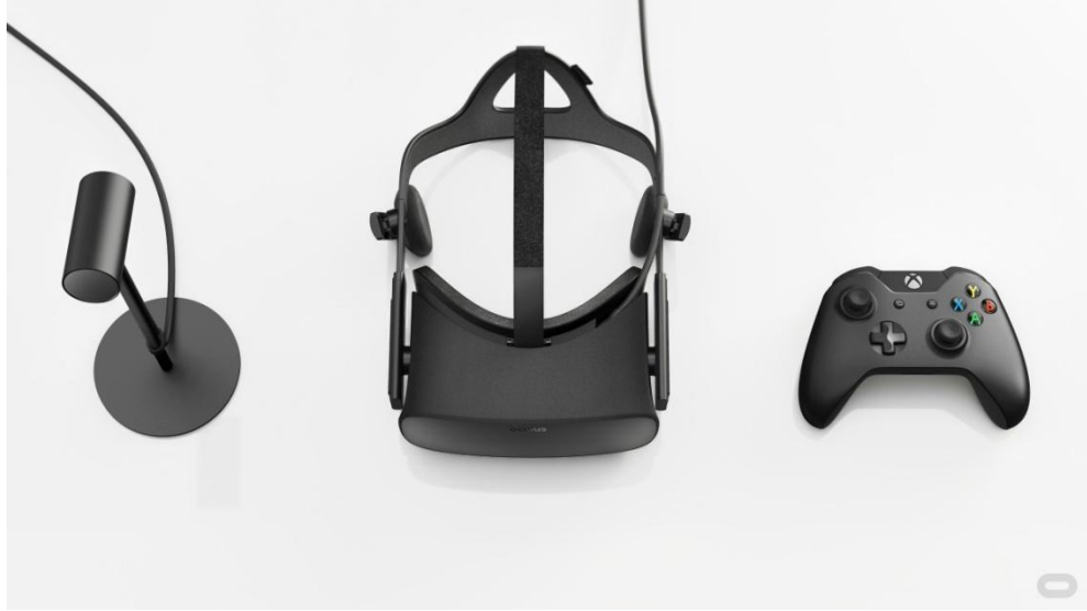
Figure 1: Oculus Constellation tracking camera, Middle, Oculus Rift HMD, Right, bundled wireless Xbox One controller (Rift)
