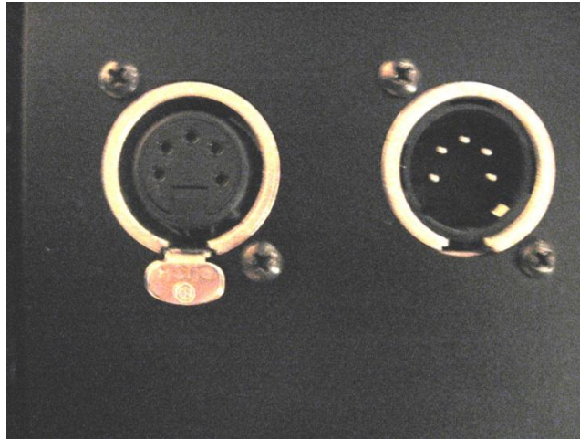
Figure 12 - Female (left) and male (right) DMX connectors
