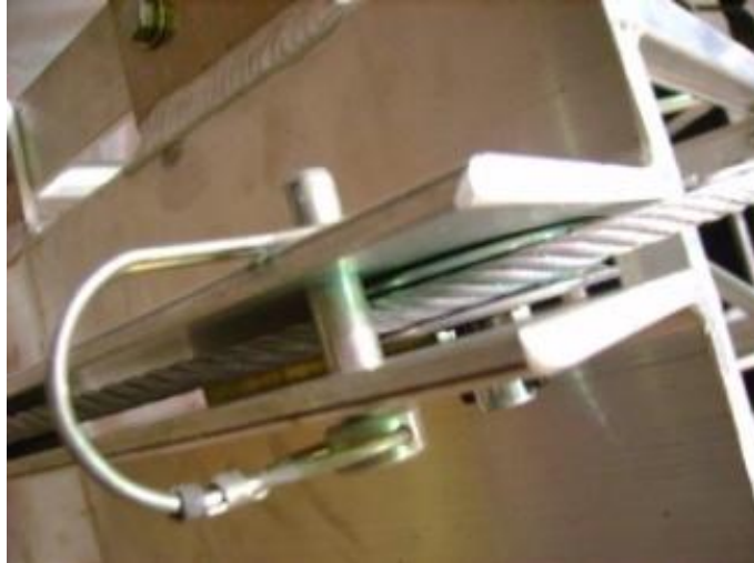
Figure 14: The aircraft cable on the pulley, and the pin holding it there
