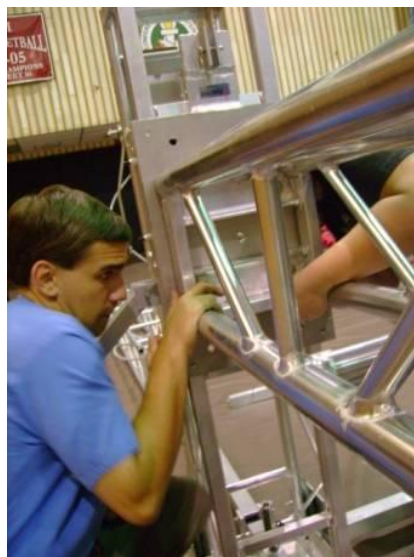
Figure 11: Attaching the truss to a slideblock
