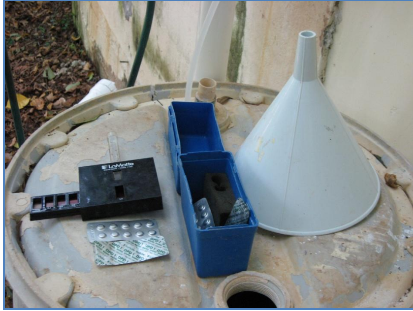
Figure A-9: Chlorine Testing Equipment
