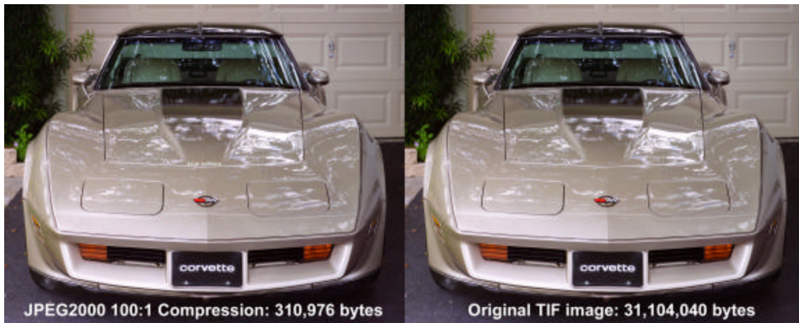
Figure 6: Comparison of storage size between JPEG2000 and TIFF
