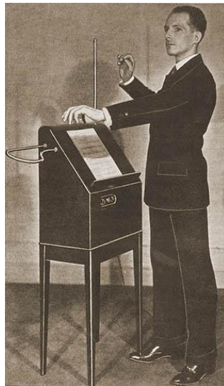
Figure 2: Leon Theremin posing with the Theremin, the left loop controls volume while the right loop controls pitch.
