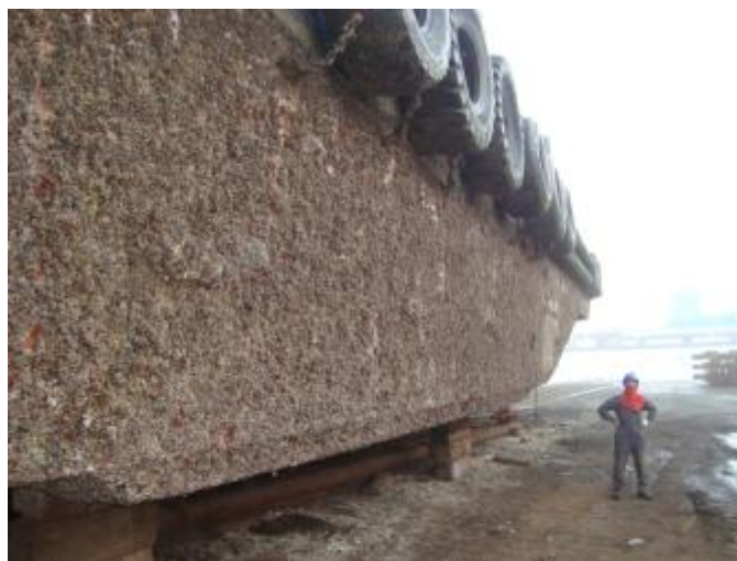
Figure 1: Biofouling on side of ship (Fathom Shipping, 2013)
