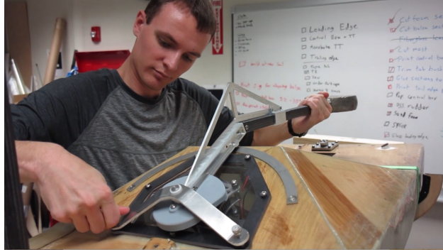
Figure 58: Hans Assembling the Movable Ballast for Testing
