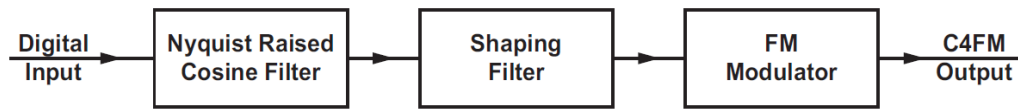
Figure 2.3: Structure of a C4FM modulator. The modulator takes in data from the digital input and multiplies it with a Nyquist raised cosine filter and a shaping filter to create four distinct lobes. Finally the signal is modulated with an FM modulator like an analog signal.
