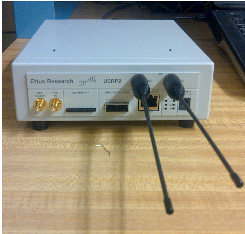
Figure 2.2: USRP2 Base with internal WBX daughtercard and dual band VHF/UHF Antennas
