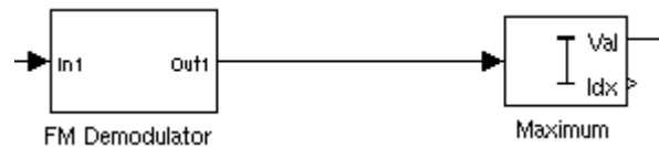
Figure 4.8: A Simulink model of an FM demodulator. Once the signal is demodulated the largest value in the frame is send to the next part of the model.
