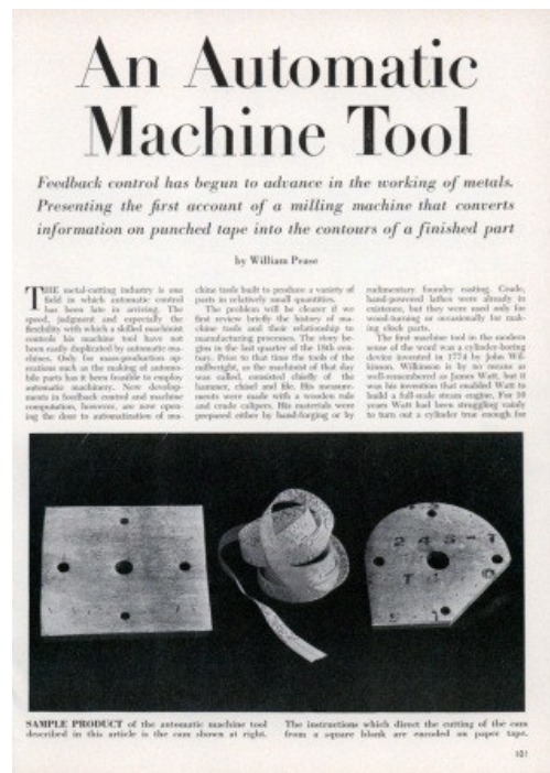
Figure 10: This article is from a 1952 issue of Scientific American (note the date relative to the advent of numerical control). The picture contained within is an excellent example of punch-tape and numerical control. One can see just how much “code” is required
