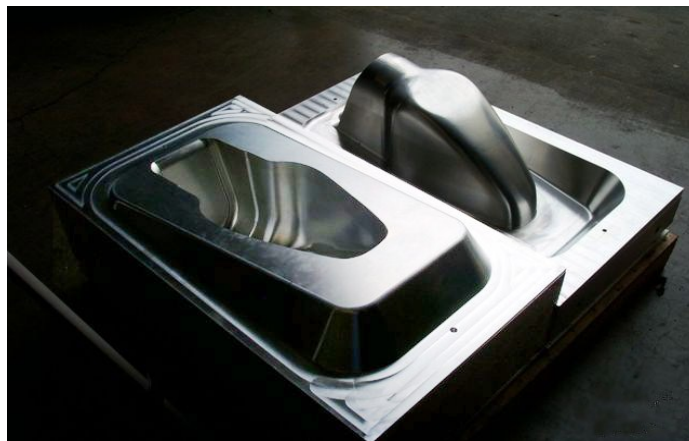
Figure 1: Example of a mold created using high-speed, 5-axis machining.
