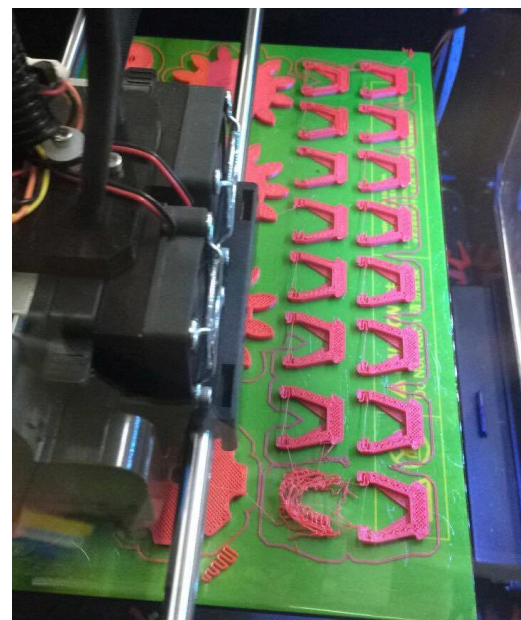
Figure 47: 3D printing a chain and sprocket
