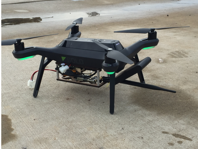
Figure 6.7: The complete system mounted on the drone. In flight testing was done with this setup.
