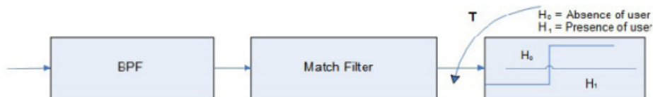
Figure 2.6: Flow diagram of matched filter. The input signal is bandpass filtered. The resulting signal is then correlated with the expected signal. If the output of this correlation passes a threshold, the signal is considered as present.
