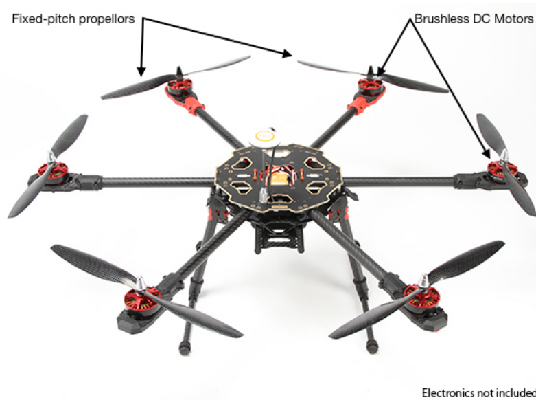
Figure 2.18: A multicopter with 6 rotors. The brushless DC motors allow for very high speeds and a high degree of control [9].
