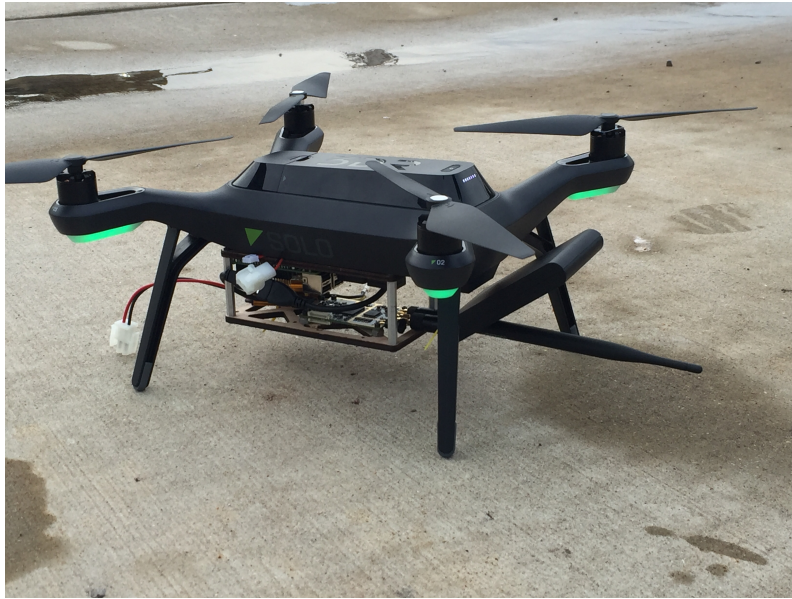
Figure 3: The complete system mounted on the drone. In flight testing was done with this setup.
