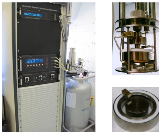
Figure 4: Dielectric relaxation spectroscopy (a), sample holder (b), and sample cell (c).
