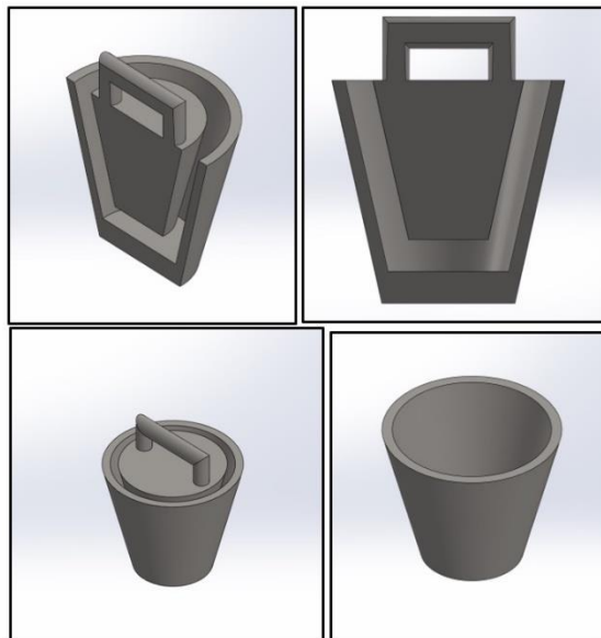
Figure 11: Model of plastic mold for ceramic piece to increase efficiency.
