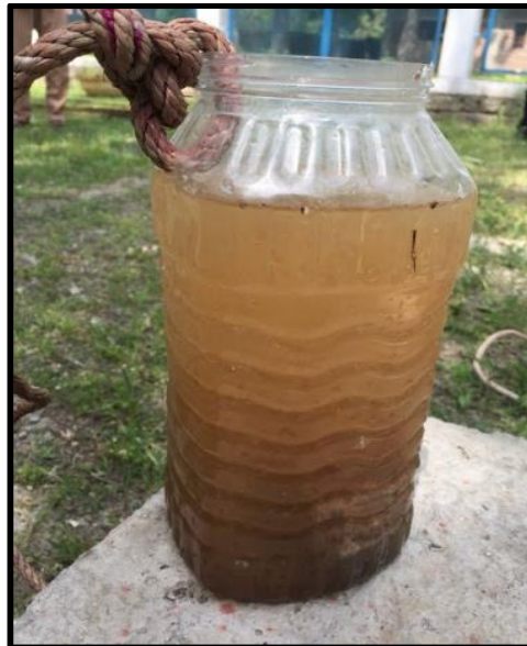
Figure 7: Water sample from a closed tap, showing possible iron contamination.
