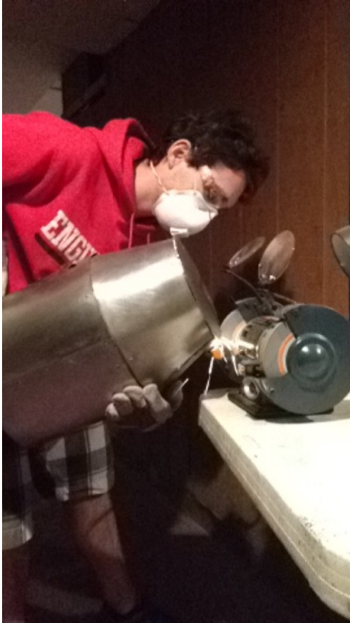
Figure 55: Using a metal grinder to smooth out edges on the helm.
