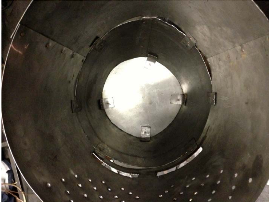
Figure 53: Top-down view of the upside-down helmet. Note the steel tabs attaching the cylinder to the frustum, and the frustum to the flat top piece.
