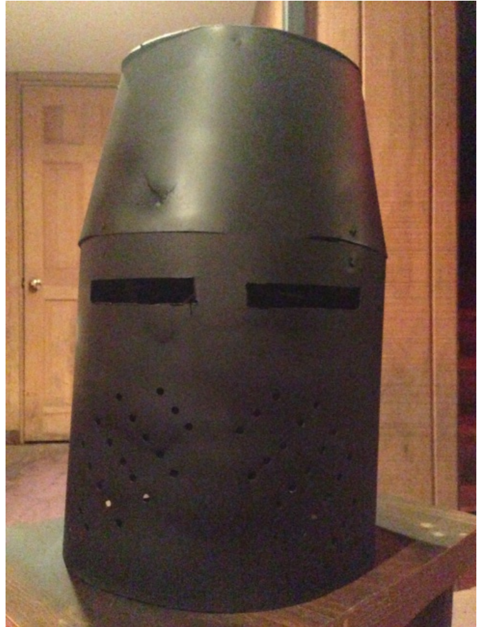
Figure 56: The helm after being coated with Rust-Oleum.
