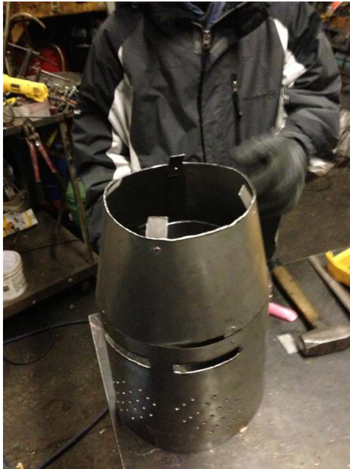
Figure 50: Frustum attached at the top of the bottom piece by copper rivets.
