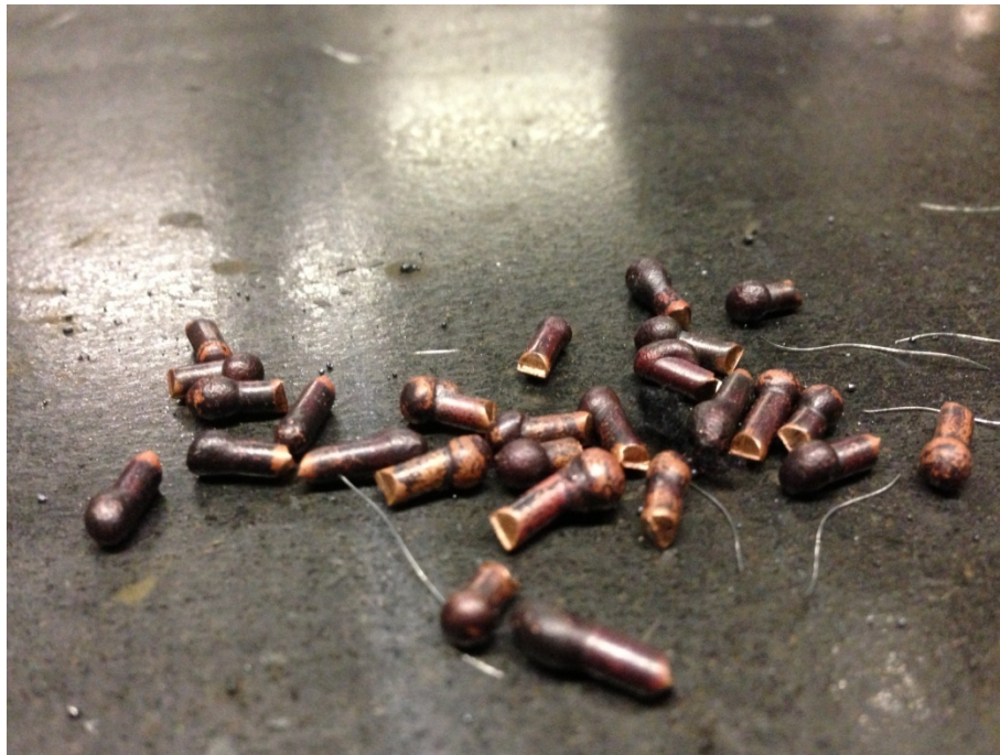
Figure 38: Copper rivets created from melting copper wire.
