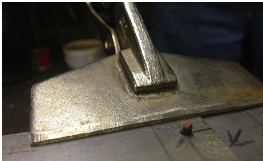
Figure 41: Copper rivet threaded through the holes in the metal pieces.
