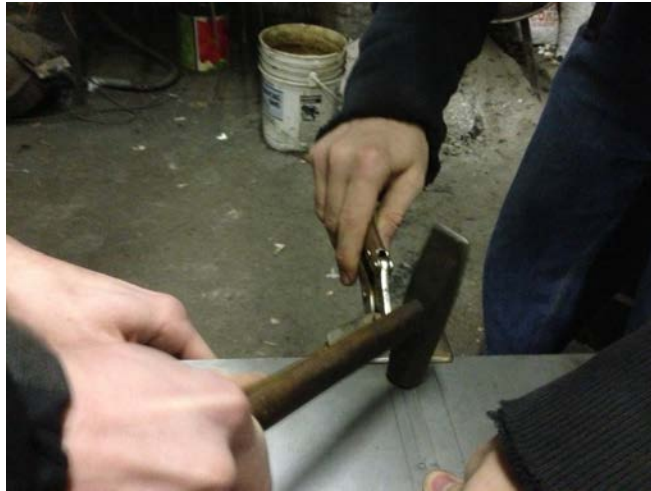
Figure 42: hammering a rivet to fasten the metal pieces together.
