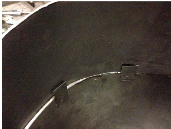
Figure 49: Steel tabs after being riveted to cylinder, but before being riveted to the frustum.
