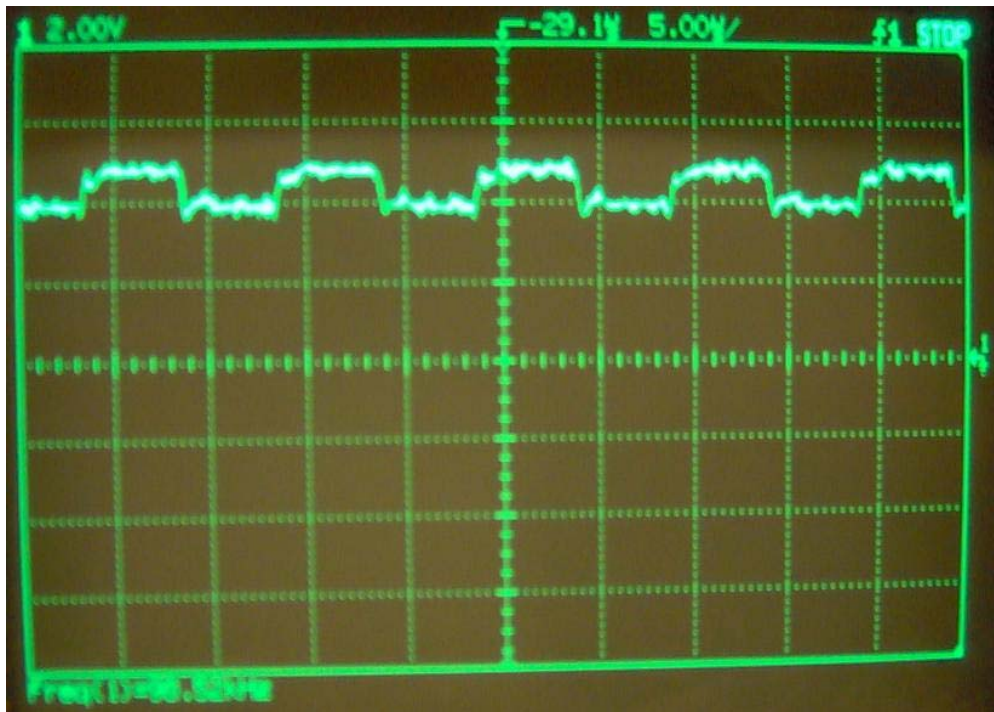
Figure 5-2 Detector Stage output Voltage (No Capacitor)
