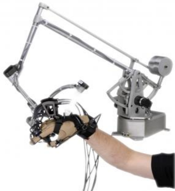
FIGURE 11: CYBERGRASP WITH ATTACHED CYBERFORCE ARMATURE BY CYBERGLOVE SYSTEMS
