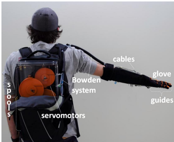
FIGURE 15: BOWDEN SYSTEM DEVELOPED BY AIM LAB IN WORCESTER POLYTECHNIC INSTITUTE
