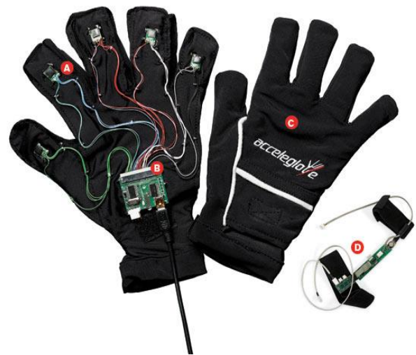
FIGURE 3: ACCELEGLOVE, A PROGRAMMABLE GLOVE THAT RECORDS HAND AND FINGER MOVEMENTS
