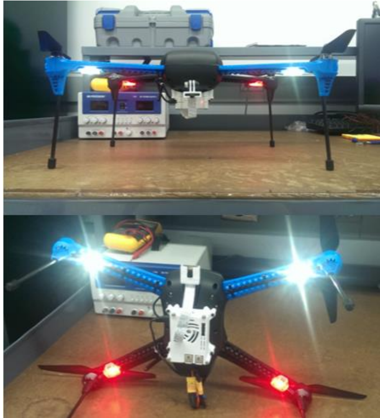
Figure 14: 3D Printed Parts Mounted on IRIS+
