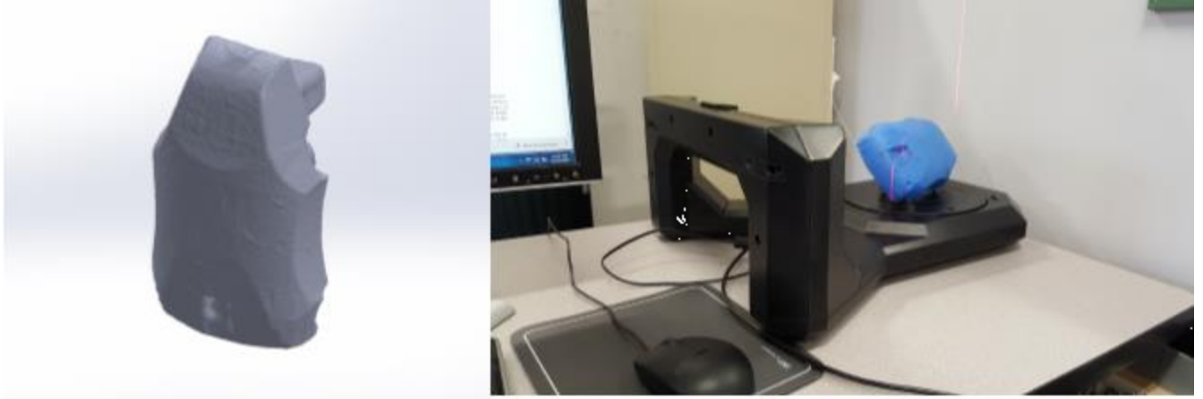
Figure 12: 3D Scanning of IRIS+ Belly
