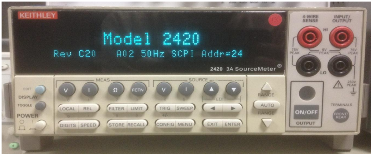
Figure 20: The Keithley Source Meter. Using LabView, this device was programmed to run a sweep on the EVAL-AD7091RSDZ board.
