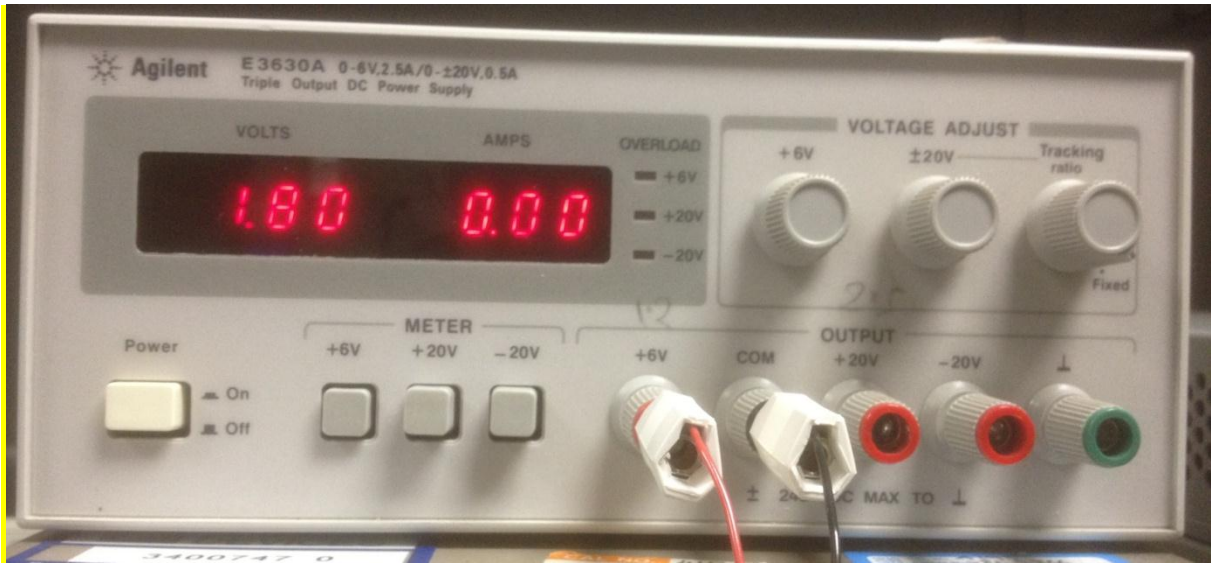
Figure 24: The Agilent Triple Output Power Supply. This is an adjustable power supply that was used to test the device under different voltage levels at VDRIVE.
