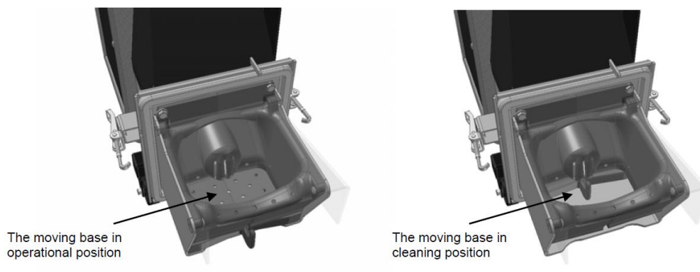
Figure 2.4: Burner Bowl Scrape Cycle 13
