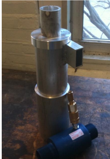
Figure 4.2: Cyclone System Prototype
