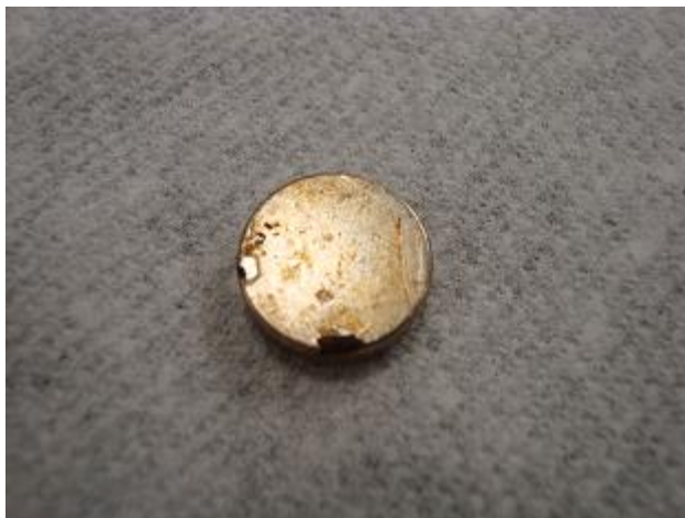
Figure 58: Magnet after it was removed from the movable arm. The nickel appears to be chipped causing it to rust.
