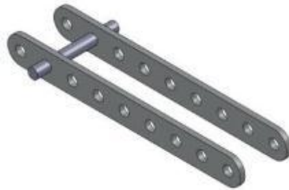
Figure 16: Pin and hole track system that was considered for adjustability of the movable arm.
