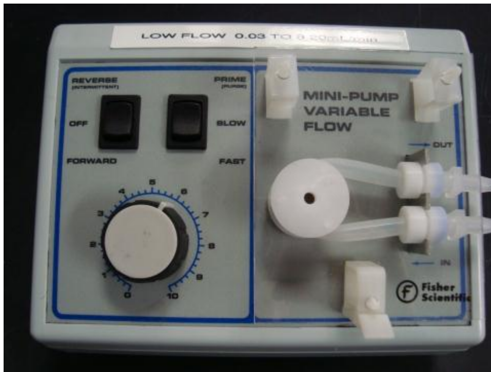
Figure 19: Fisher Scientific Variable-Speed Pump Low Flow was used to pump fluid through the bioreactor. Flow rates ranged from 0.003-8.20mL/min.
