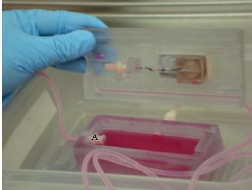
Figure 41: After two days in the incubator and a minor leak, the remaining media in the bioreactor filled the chamber to about the middle of the inlet Luer (A).
