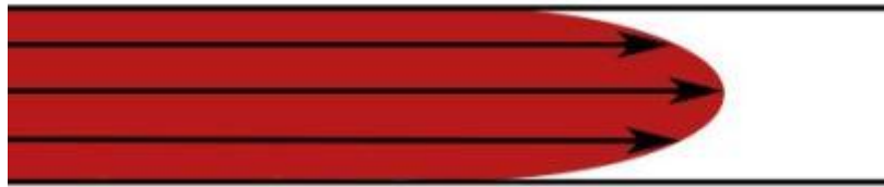
Figure 1: Schematic of a laminar flow profile. Particles flow parallel to the vessel walls and those in the center of the vessel have a higher velocity.
