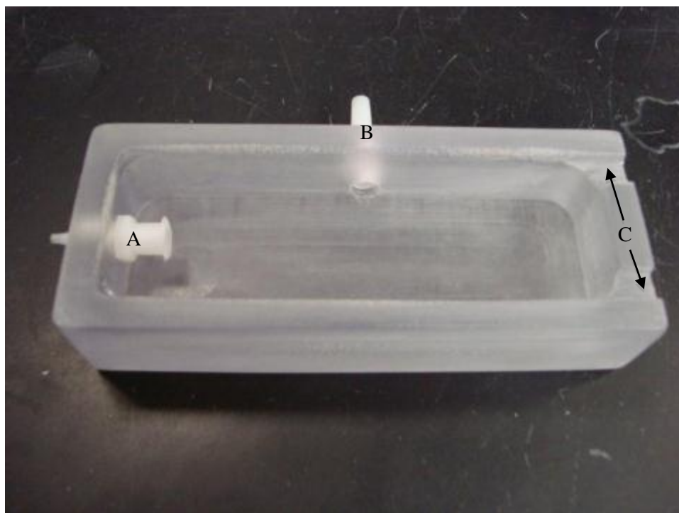
Figure 27: Final design chamber showing female inlet Luer (A), male outlet Luer (B), and slots for ridges on lid (C).
